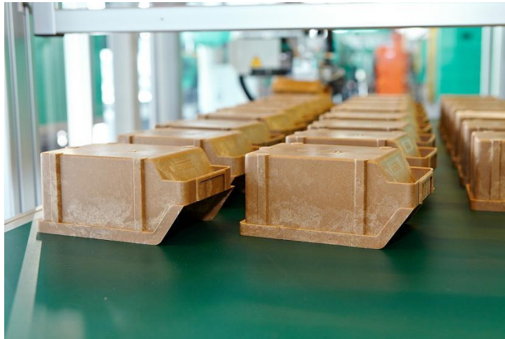
Fig. 8. Injection molded biocomposite. (Source: https://www.arburg.com/en/solutions/by-technology/special-injection-moulding-processes/ ). Used with permission from Arburg Company Press
