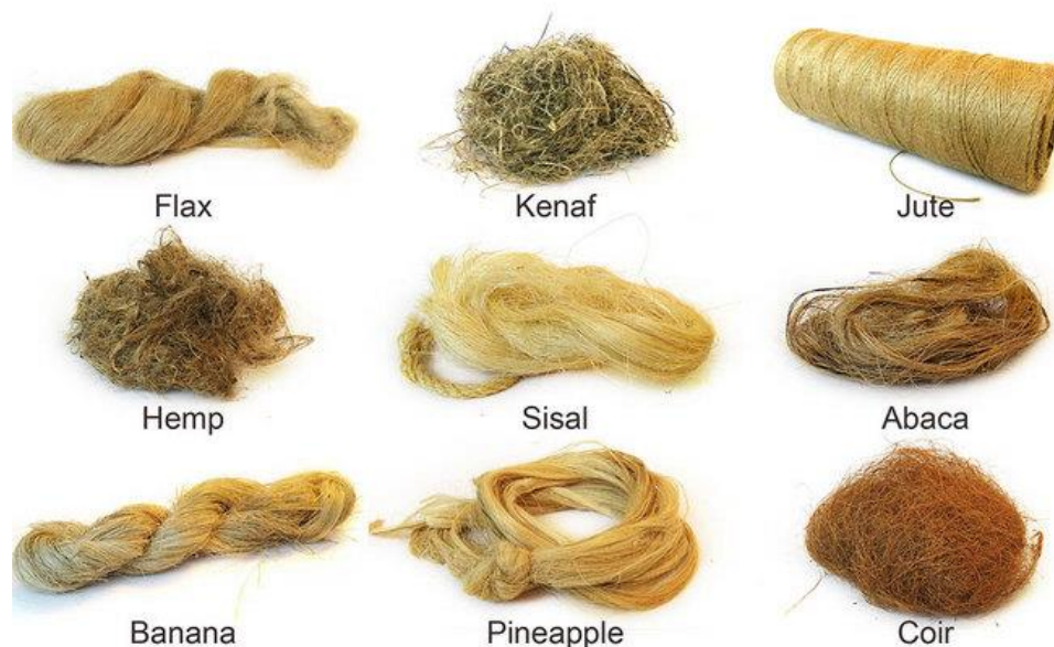
Fig. 5. Some industrially used plant fibers. (Source: Nurazzi et al. 2021, Polymers 13, 646. Creative Commons BY 4.0)
