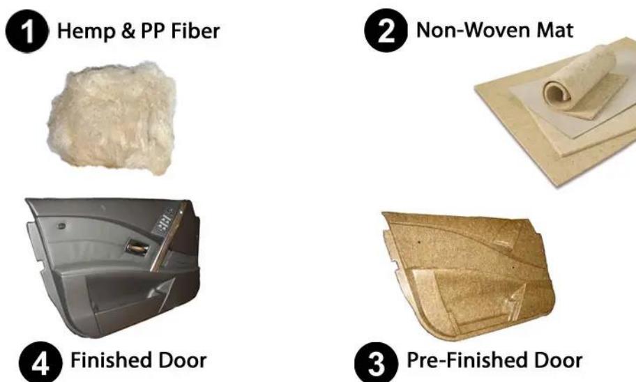
Fig. 7. Hot press molding of non-woven hemp-pp composites used in manufacture of the door of the car. (Source: https://www.globalhemp.com/blog/automotive-composites/ ). Used with permission from Global Hemp Company
