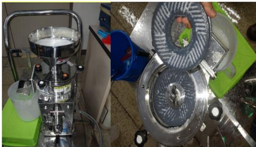
Fig. 9. Masuko Sangyo Super Masscolloider grinder for nanocellulose production. The photos were taken by N. Ayrlimis.
