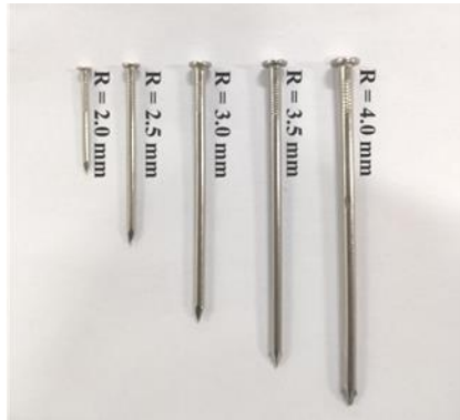
Fig. 1. The round steel nails used for nail-holding power test
