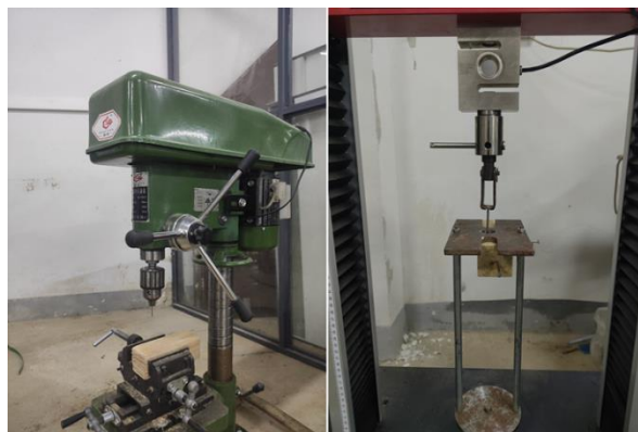
Fig. 3. The test of nail-holding power
