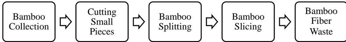
**Fig. 3.** Bamboo fiber preparation steps
