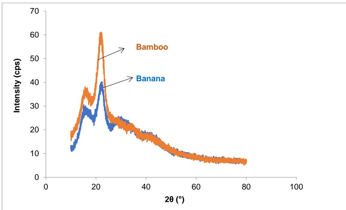
**Fig. 6.** X-ray diffraction analysis of banana and bamboo fibers
