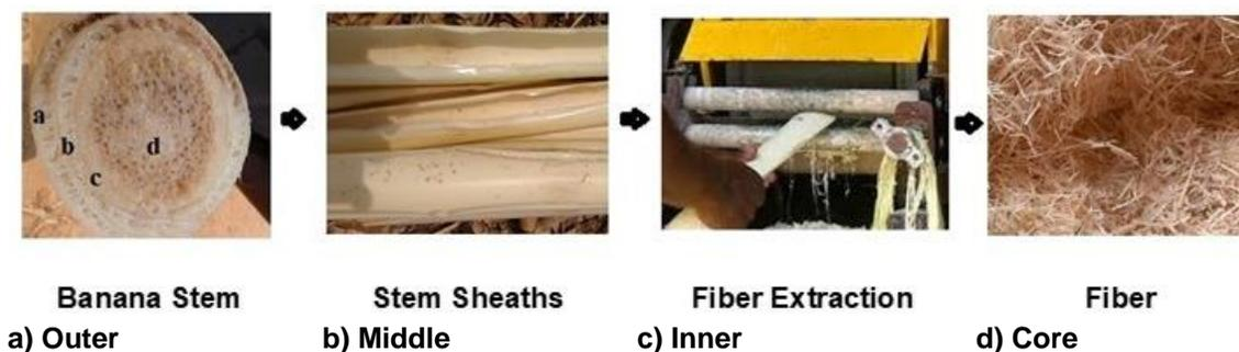
Fig. 2. Sequential images of banana fiber preparation
