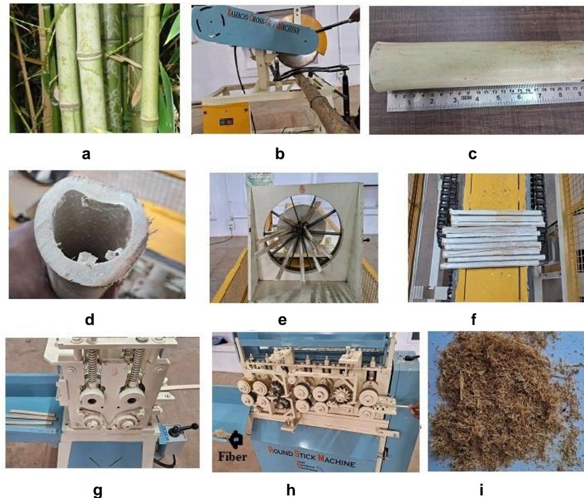
**Fig. 4.** (a) Bamboo plants, (b) bamboo cutting machine, (c) culm length, (d) culm top view, (e) bamboo culm splitting, (f) split culm, (g) slicing machine, (h) bamboo stick making, (i) fiber waste
