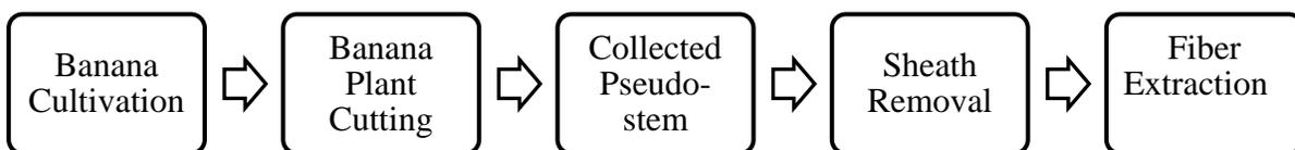
Fig. 1. Banana fiber preparation steps
