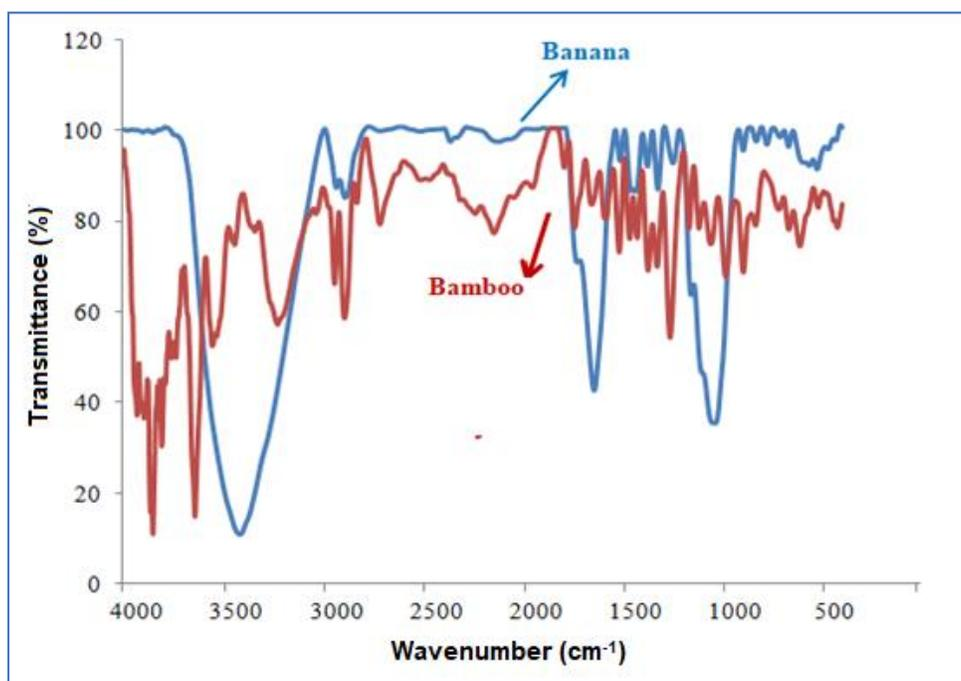
Fig. 7. FTIR analysis of banana and bamboo fibers
