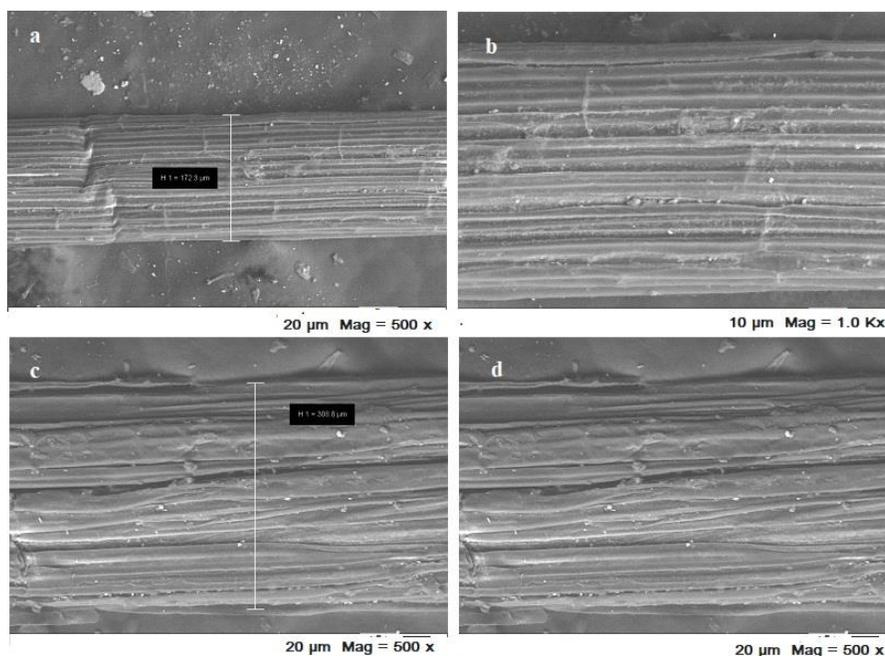
**Fig. 5.** SEM analysis of (a and b) banana and (c and d) bamboo fibers
