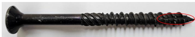
Fig. 7. Processing tip of Korea STS fastener (Type D)
