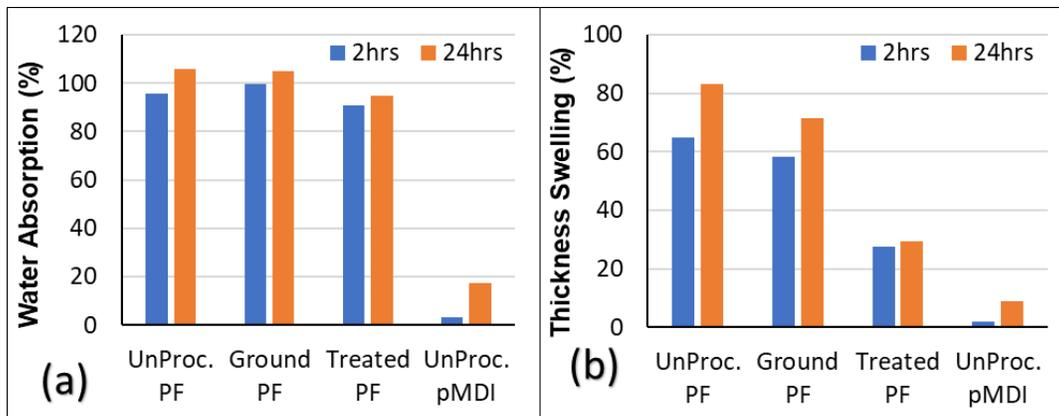
Fig. 5. (a) Water absorption and (b) thickness swelling results of rice-husks board
