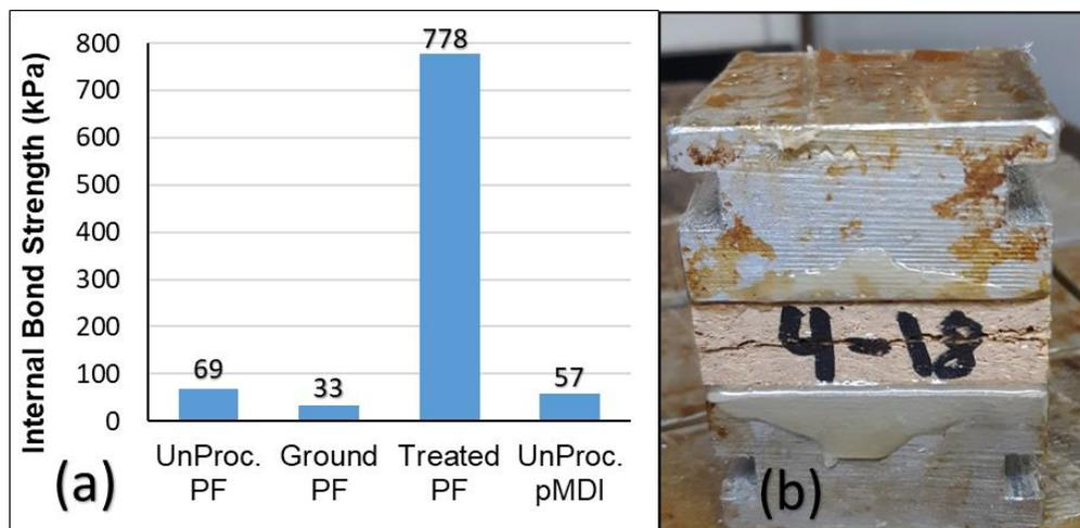
Fig. 4. (a) Internal bond strength of fabricated rice husk composite boards and (b) failure mode of IB specimens
