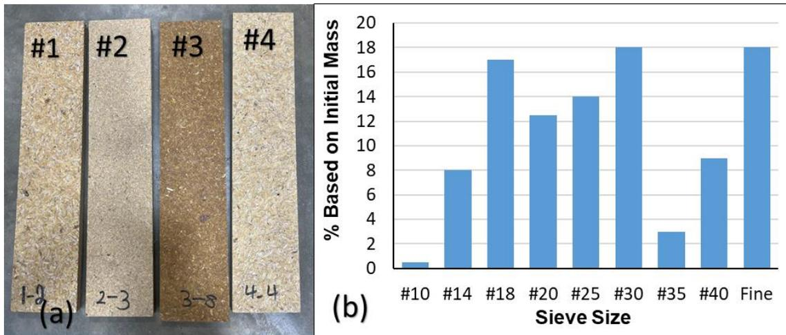
**Fig. 2.** (a) Fabricated rice husk boards: #1: unprocessed rice husks+PF, #2: ground+PF, #3: treated+PF, and #4: unprocessed +pMDI, and (b) sieve analysis of ground rice husks.
