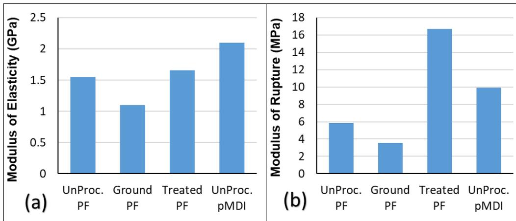
Fig. 3. Bending test results (a) modulus of elasticity and (b) modulus of rupture
