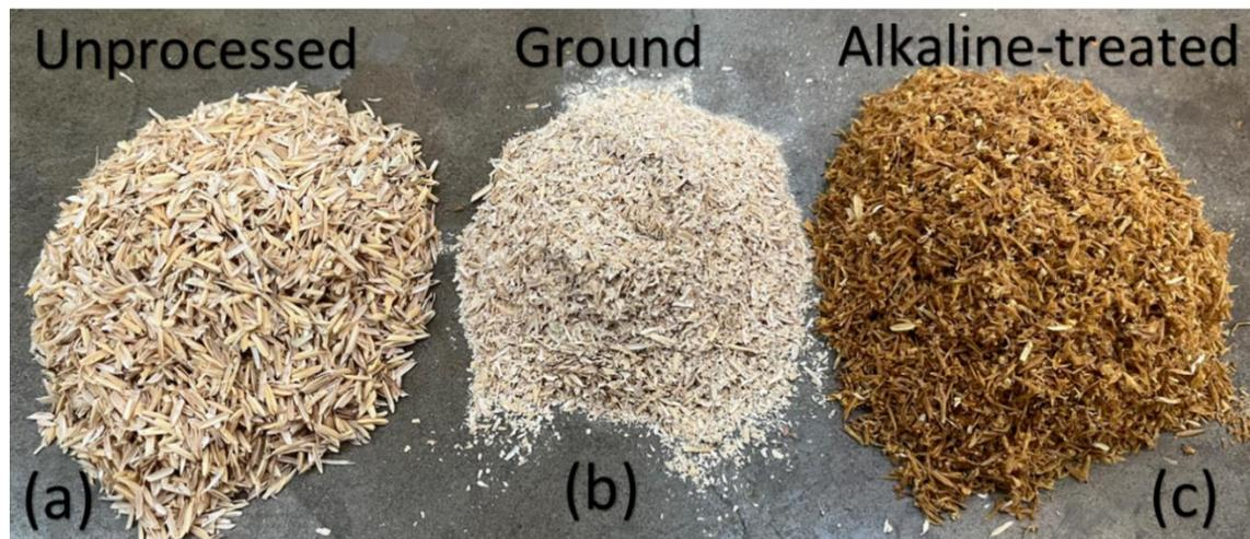
Fig. 1. Raw materials: (a) unprocessed, (b) ground, and (c) alkaline treated rice husks
