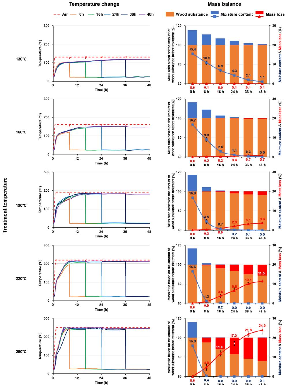
**Fig. 2.** Changes in air temperature (left) and in the mass balance of thermally modified wood (right)
