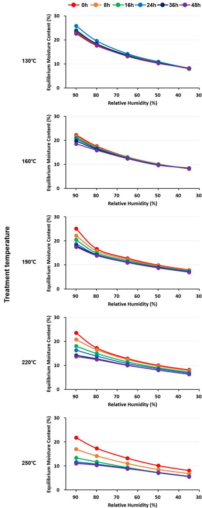
Fig. 3. Desorbed equilibrium moisture content of thermally modified wood
