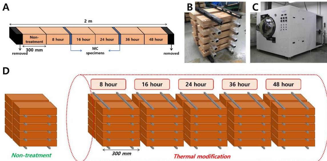
**Fig. 1.** Preparation of wood specimens for thermal modification. A. specimen preparation method for one lumber; B. specimen bundled with wire rope; C. thermal modification equipment; D. specimen bundles stacked in the reactor
