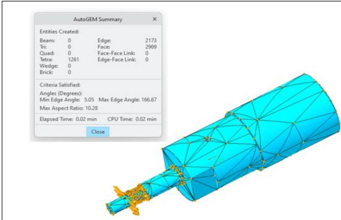
**Fig. 10.** AutoGem – meshing of finished elements
