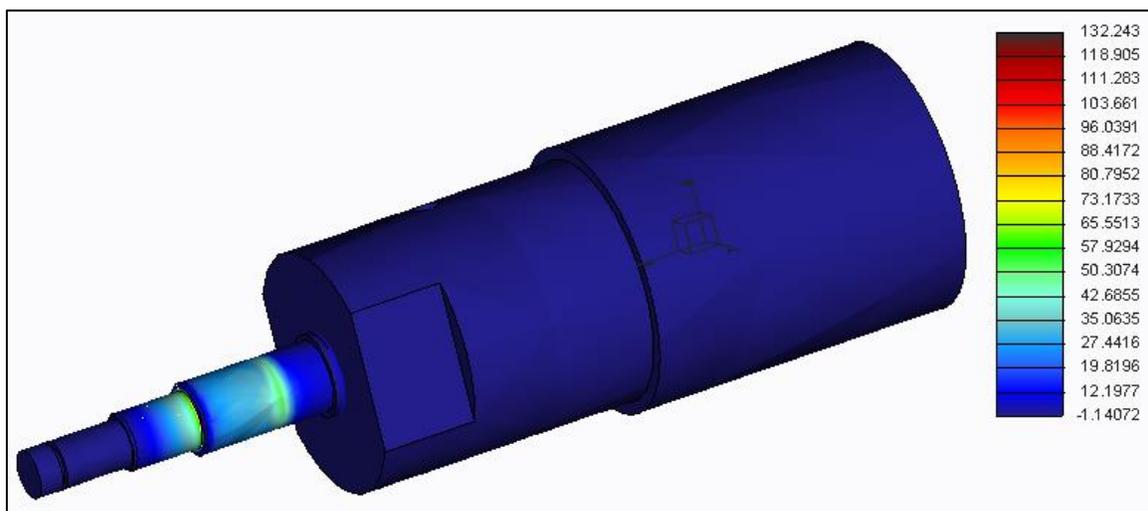
**Fig. 11.** Shaft stress analysis
