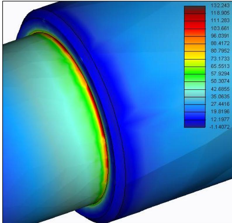
**Fig. 12.** Detail of the area under the most stress
