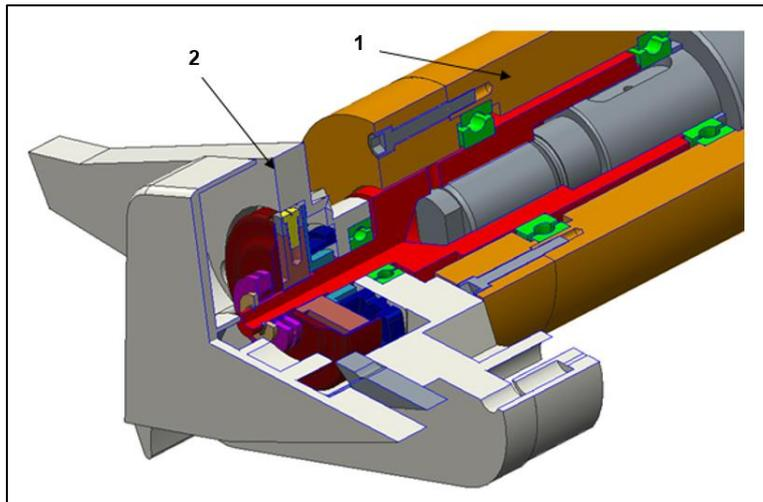
**Fig. 2.** Model of the fixture for holding the cutting mechanism in the cut
