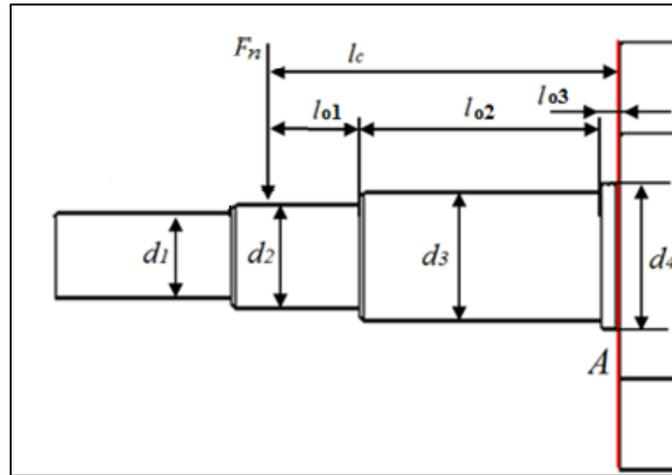
**Fig. 6.** Loaded part of the shaft
