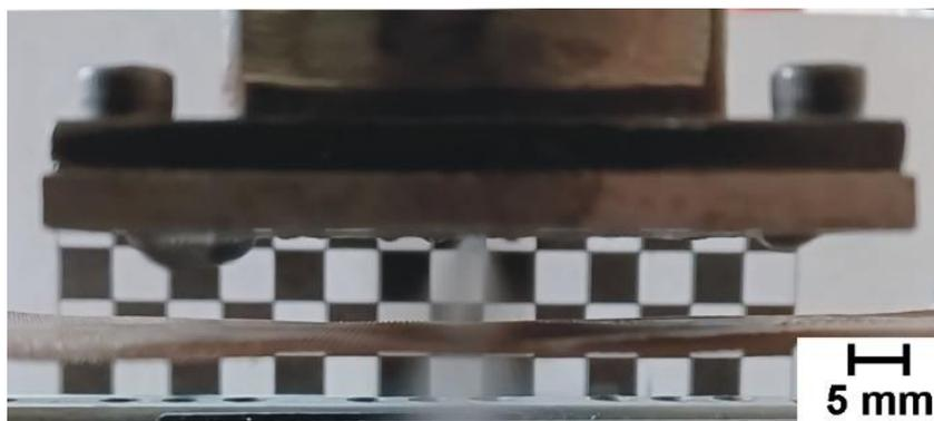
**Fig. 2.** Photograph showing the shape of the air jet flowing from the nozzle of the head
