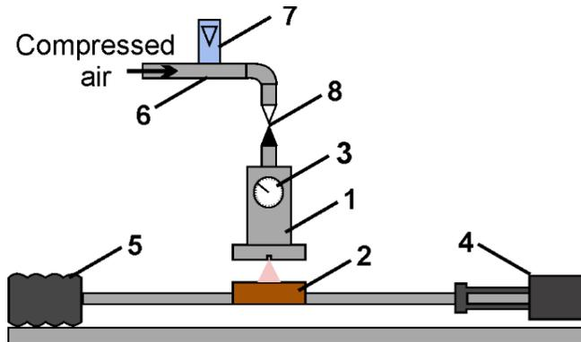
**Fig. 1.** Schematic diagram of the research stand. 1 - head, 2 - trolley with sample, 3 - manometer, 4 - drive system, 5 - trolley energy absorption system, 6 - pipeline, 7 – rotameter, 8 – valve
