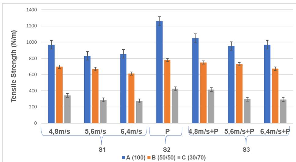
**Fig. 4.** Tensile strength for samples cut from a formed sheet in the MD direction, for all study series
