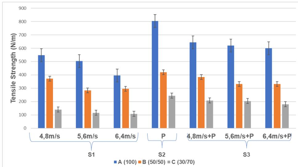
Fig. 5. Tensile strength for samples cut from a formed sheet in the CD direction, for all study series
