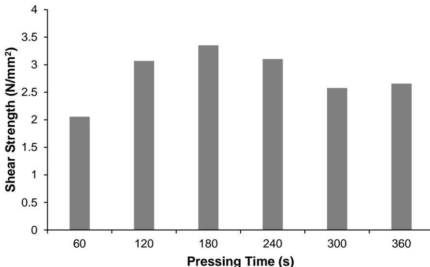
**Fig. 3.** Shear strength of MUF adhesive joint between two beech veneers for determining the optimal pressing time at a pressing temperature of 180°C
