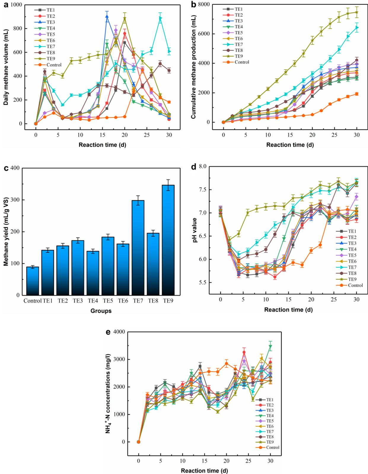
**Fig. 2.** Performances of batch AD of KW with varying TEs supplementation strategies. Daily methane volume (a), cumulative methane production (b), methane yield (c), pH (d) and  $\text{NH}_4^+\text{-N}$  (e)
