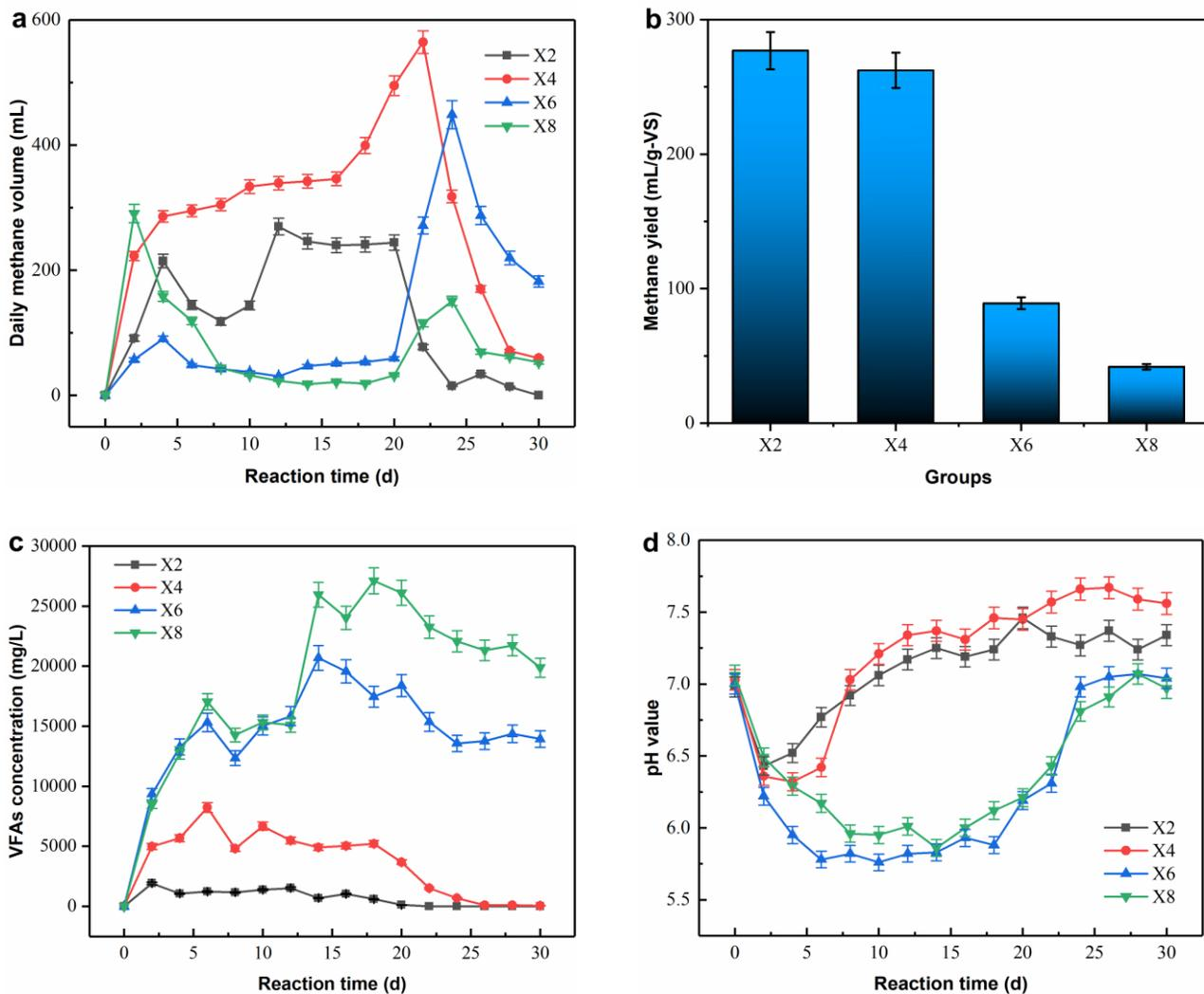
**Fig. 1.** Performances of batch AD of KW at different organic loadings conditions. Daily methane volume (a), methane yield (b), VFAs concentration (c), and pH (d)
