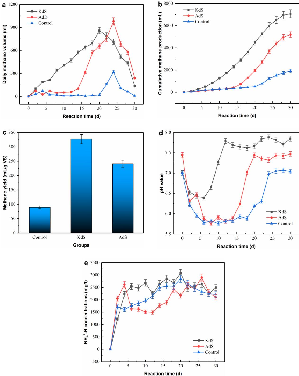
**Fig. 4.** Performances of batch AD of KW with the application of domesticated sludge by KW and HAc as inoculum. Daily methane volume (a), cumulative methane production (b), methane yield (c), pH (d) and  $\text{NH}_4^+\text{-N}$  (e)
