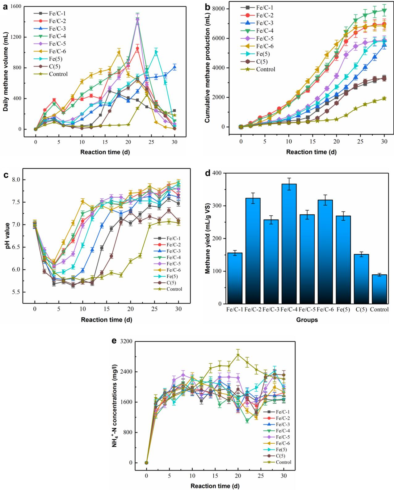
**Fig. 3.** Performances of batch AD of KW with varying ZVI/PAC supplementation strategies. Daily methane volume (a), cumulative methane production (b), pH (c), methane yield (d), and  $\text{NH}_4^+\text{-N}$  (e)
