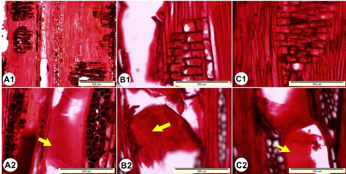
**Fig. 6.** Radial sections of *Entandrophragma* species. *Entandrophragma cylindricum*; (A1) rays in radial section; (A2) numerous, small inter-vessel pits (arrow); *Entandrophragma utile*; (B1) heterogenous rays; (B2) numerous, small inter-vessel pits (arrow); *Entandrophragma angolense*; (C1) heterogenous rays; (C2) numerous, small inter-vessel pits (arrow). Scale bars: A1= 500 µm; A2, B1, B2, C1, C2=200 µm
