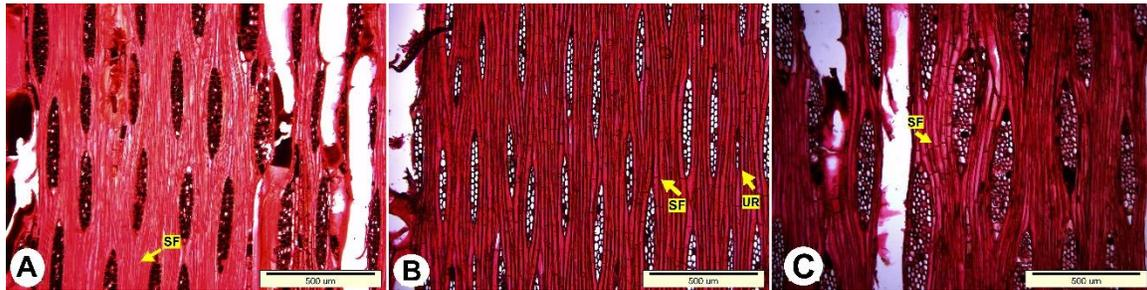
**Fig. 8.** Tangential section of *Entandrophragma* species. (A) *E. cylindricum*; (B) *E. utile*; (C) *E. angolense*. (SF) septate fibre; (UR) uniseriate ray. Scale bars: 500 µm
