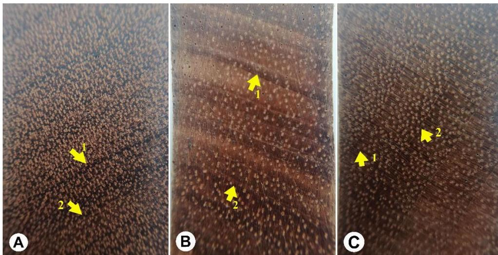
**Fig. 2.** Macroscopic views of *Entandrophragma* species. (A) *E. cylindricum*, a narrow zone of denser fibrous tissue (arrow 1), marginal parenchyma bands (arrow 2); (B) *E. utile*, a narrow zone of denser fibrous tissue (arrow 1), marginal parenchyma bands (arrow 2); (C) *E. angolense*, a narrow zone of denser fibrous tissue (arrow 1), marginal parenchyma bands (arrow 2) (Hand lens adapted to mobile phone, 10x)
