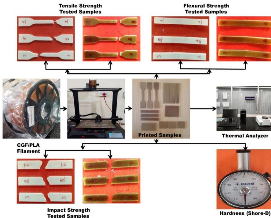
Fig. 1. Schematic diagram of the process adopted
