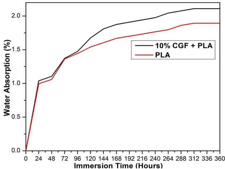
Fig. 9. Water absorption behaviors of PLA and 10 wt.% CGF/PLA filament composite
