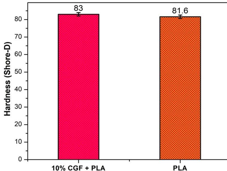
**Fig. 6.** Hardness of PLA and 10 wt% CGF/PLA filament composite (Error bar represents 95% confidence interval of the mean.)
