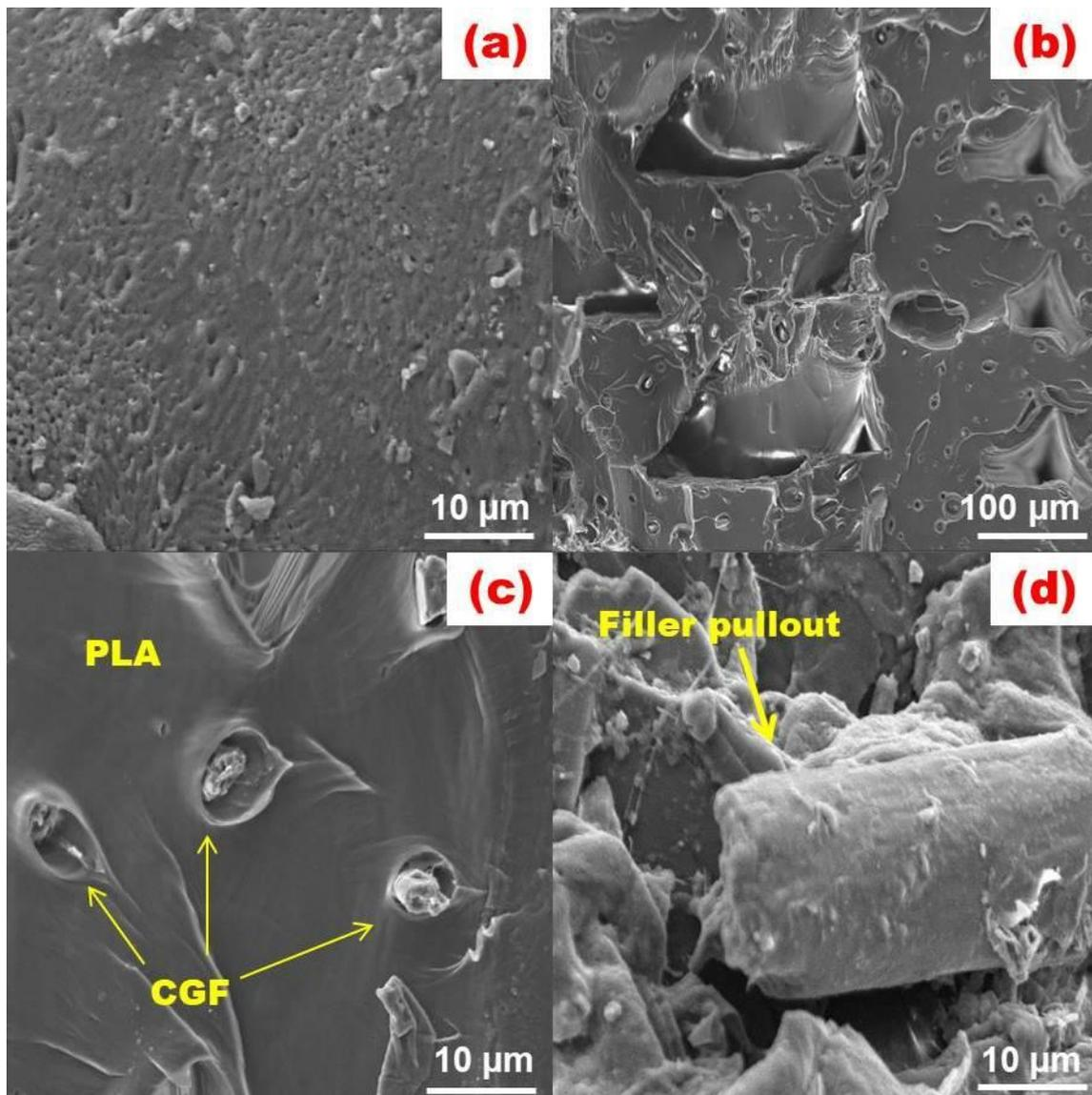
Fig. 7. SEM images of (a) Pure PLA (b - d) 10 wt% CGF/PLA filament composite
