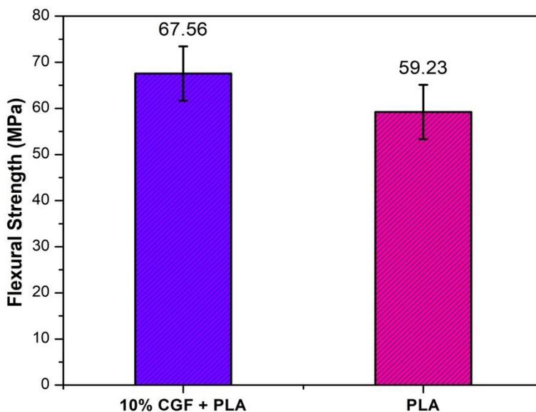
**Fig. 4.** Flexural strengths of PLA and 10 wt% CGF/PLA filament composite (Error bar represents 95% confidence interval of the mean.)
