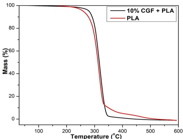
**Fig. 8.** TGA curves of PLA and 10 wt% CGF/PLA filament composite
