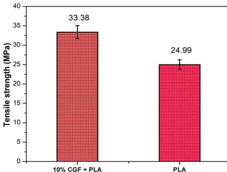
**Fig. 3.** Tensile strengths of PLA and 10 wt% CGF/PLA filament composite (Error bar represents 95% confidence interval of the mean)
