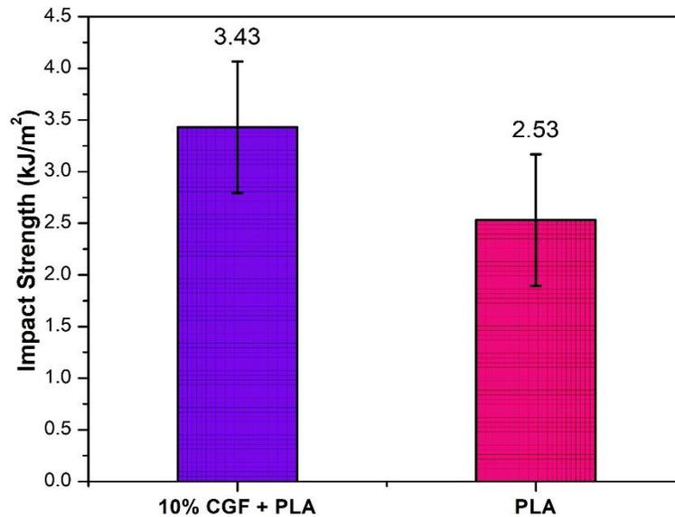
**Fig. 5.** Impact strengths of PLA and 10 wt% CGF/PLA filament composite (Error bar represents 95% confidence interval of the mean.)
