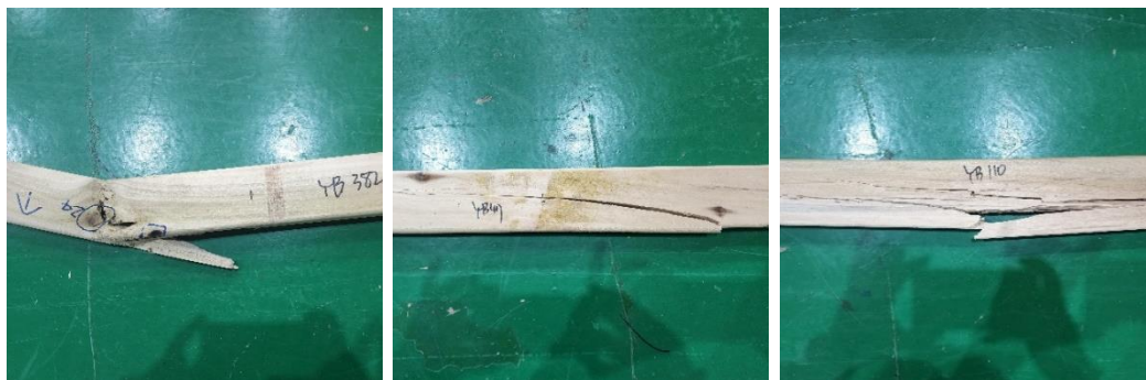
Fig. 4. Failure modes in bending test (from left: knot, grain angle, and tension)
