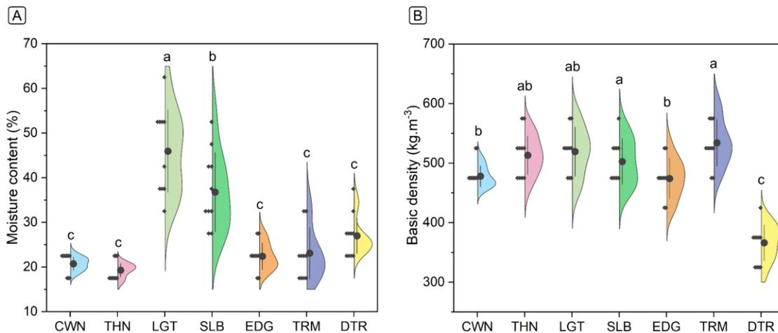
**Fig. 2.** Physical attributes of the different teak wastes: (A) moisture content (%) and (B) basic density ( $\text{kg}\cdot\text{m}^{-3}$ )
