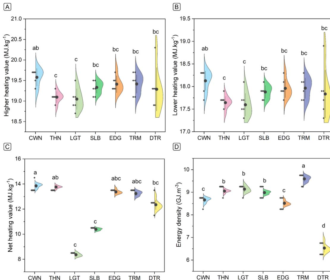
**Fig. 4.** Estimated energy attributes for the different teak wastes, where (A) higher heating value ( $\text{MJ.kg}^{-1}$ ), (B) lower heating value ( $\text{MJ.kg}^{-1}$ ), (D) net heating value ( $\text{MJ.kg}^{-1}$ ), and (E) energy density ( $\text{GJ.m}^{-3}$ )
