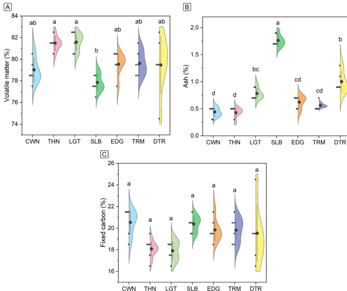
**Fig. 3.** Proximate analysis of the different teak wastes: (A) volatile matter (%), (B) ash (%), and (C) fixed carbon (%)
