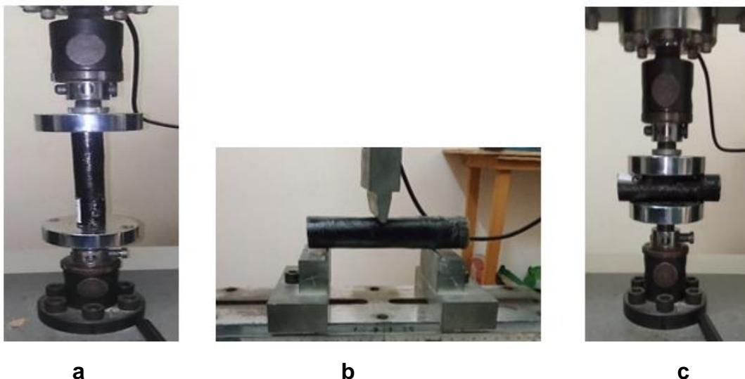
**Fig. 2.** Specimens for crashworthiness test – a: Axial compression test, b: Transverse Compression (Flexural) Test; and c: Radial compression test
