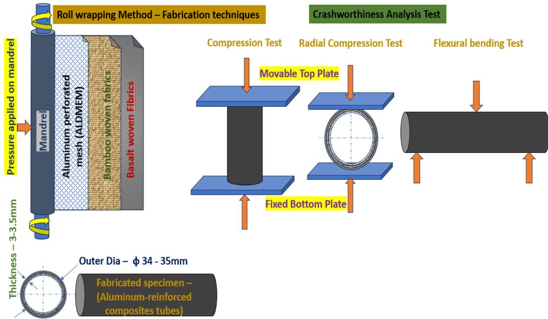
**Fig. 1.** Fabrication techniques and testing specimens
