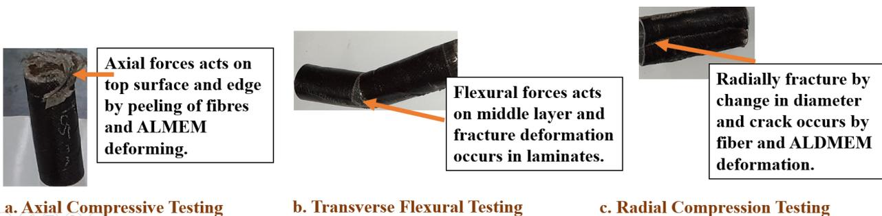
**Fig. 3.** Failure of HSS tube in three test analysis
