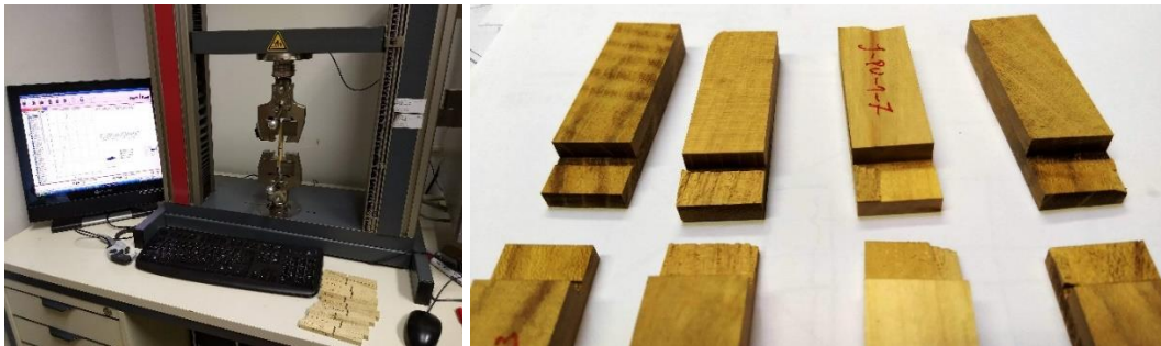
Fig. 1. Shear strength testing on universal testing machine (left) and visual evaluation of shear area percentage of wood failure after test (right) - outside samples- Robinia pseudoacacia and inner samples - Acer negundo
