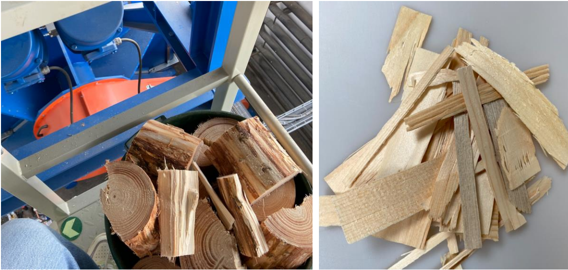
Fig. 10. Detail of the spruce specimen (a) and disintegrated strands (b) at knife ring flaker MRZ 1400
