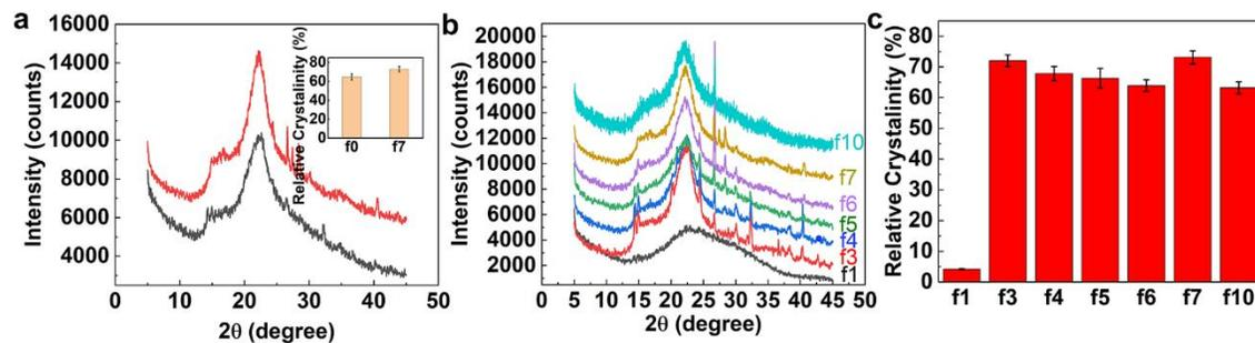
**Fig. 6.** (a) The XRD results of bio-composite f7 prior to (black curve) and after (red curve) hot-pressing. The inset depicts the relative crystallinity of bio-composite f7 prior to (f0) and after heat compression (f7). The condition f0 denotes the raw material for the preparation of bio-composite f7 prior to hot-pressing. (b) The XRD results of bio-boards f1, f3 to f7, and f10 after heat compression. (c) The relative crystallinity of bio-boards f1, f3 to f7, and f10 after heat compression
