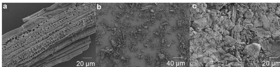
**Fig. 2.** SEM micrographs of the cross-sections of (a) corn stalk powder at a magnification of 500x, (b) *P. ostreatus* substrate powder at a magnification of 200x, and (c) f7 bio-composite at a magnification of 500x
