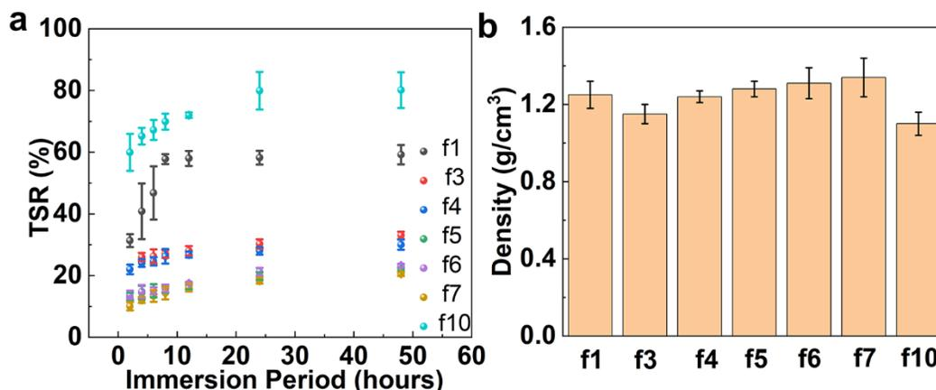
**Fig. 3.** (a) TSR values of the bio-board f1, bio-composites f3–f7, and bio-board f10 as a function of immersion period. (b) Densities of bio-board f1, bio-composites f3–f7, and bio-board f10 after hot-pressing.
