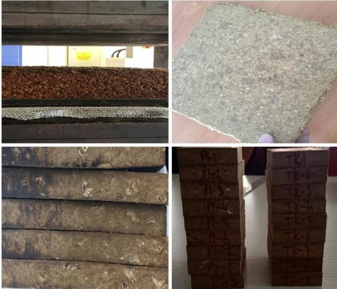
**Fig. 2.** Fiberboard mat formation, mycelium-based fiberboard, and test samples
