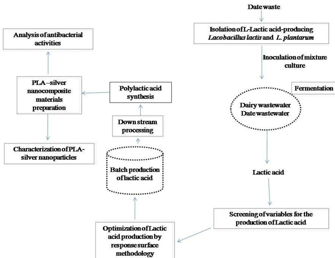
**Fig. 1.** PLA-silver nanocomposite materials preparation, analysis of composite materials and antimicrobial properties
