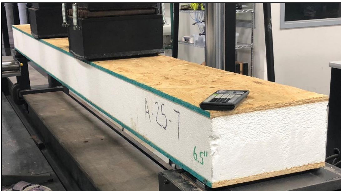
Fig. 1. Exemplar full-scale 16.5 cm (6.5 in) deep SIP test specimen in the 1/3-point test fixture
