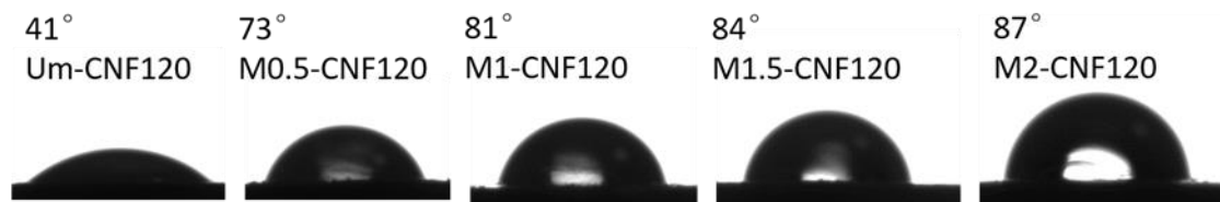
Fig. 4. Water contact angle of Um-CNF and M-CNF
