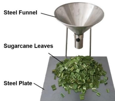
Fig. 5. Injecting funnel method to measure the stacking angle
