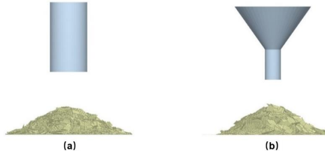
Fig. 7. Simulated accumulation angle of sugarcane leaf: (a) cylinder lifting test; (b) injection funnel test
