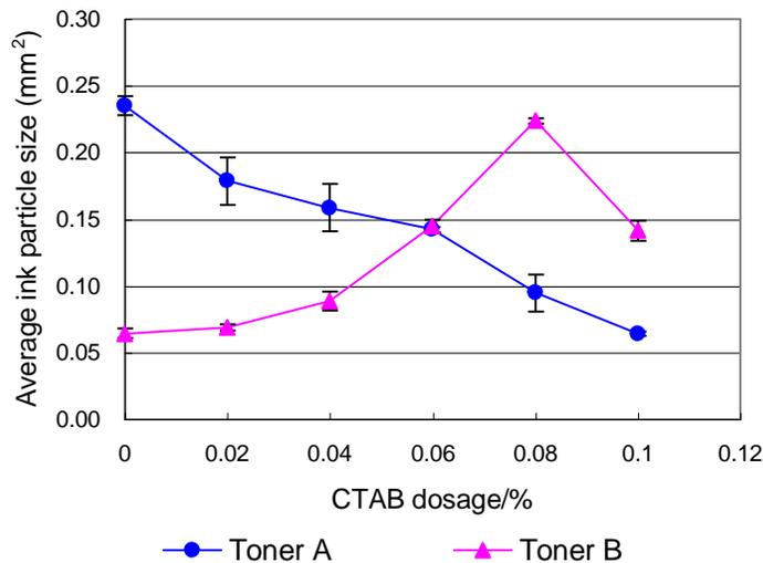
**Fig. 2.** Effect of CTAB on average ink particle size after agglomeration with 2.0% 1-octadecanol
