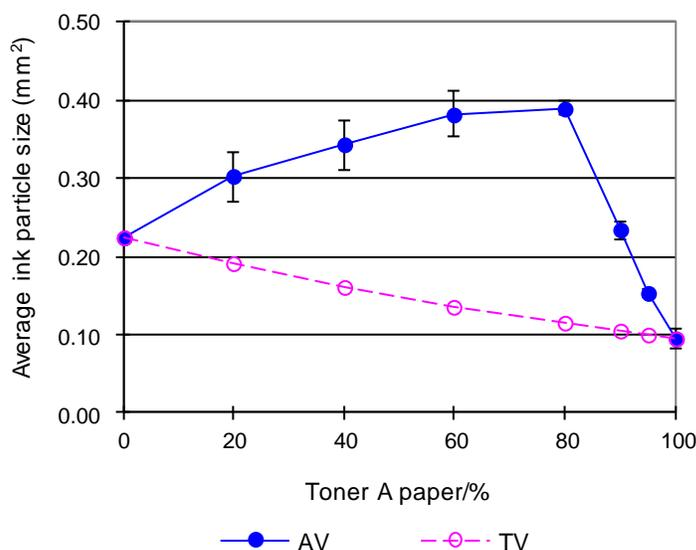
**Fig. 6.** Effect of 0.08% CTAB on average ink particle size after agglomeration of two toners mixed with different percentages at 2.0% 1-octadecanol
