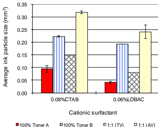
**Fig. 10.** Effect of LDBAC and CTAB on average ink particle size after agglomeration of two toners mixed by the ratio of 1:1 with 2.0% 1-octadecanol
