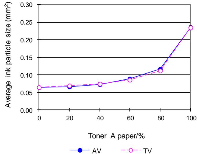
**Fig. 4.** Effect of 2.0% 1-octadecanol on average ink particle size after agglomeration of two toners mixed with different percentages
