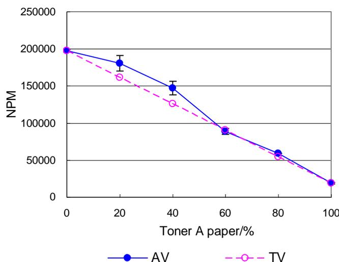
**Fig. 3.** Effect of 2.0% 1-octadecanol on NPM after agglomeration of two toners mixed with different percentages
