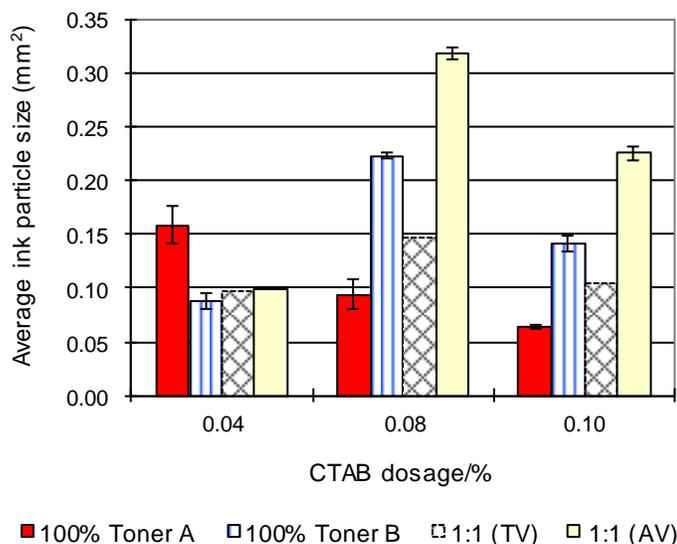
**Fig. 8.** Effect of CTAB on average ink particle size after agglomeration of two toners mixed by the ratio of 1:1 with 2.0% 1-octadecanol
