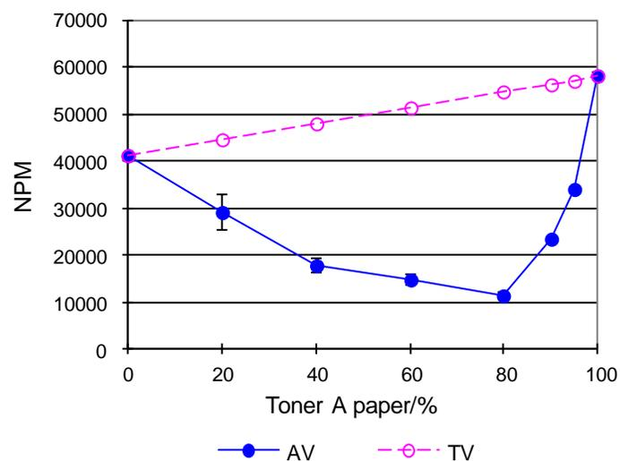
**Fig. 5.** Effect of 0.08% CTAB on NPM after agglomeration of two toners mixed with different percentages at 2.0% 1-octadecanol
