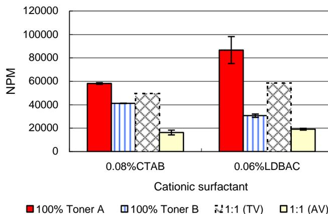
**Fig. 9.** Effect of LDBAC and CTAB on NPM after agglomeration of two toners mixed by the ratio of 1:1 with 2.0% 1-octadecanol
