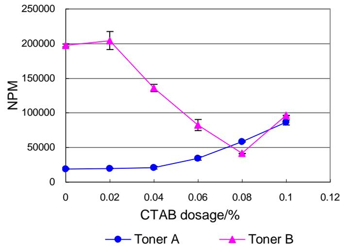
**Fig. 1.** Effect of CTAB on NPM after agglomeration with 2.0% 1-octadecanol
