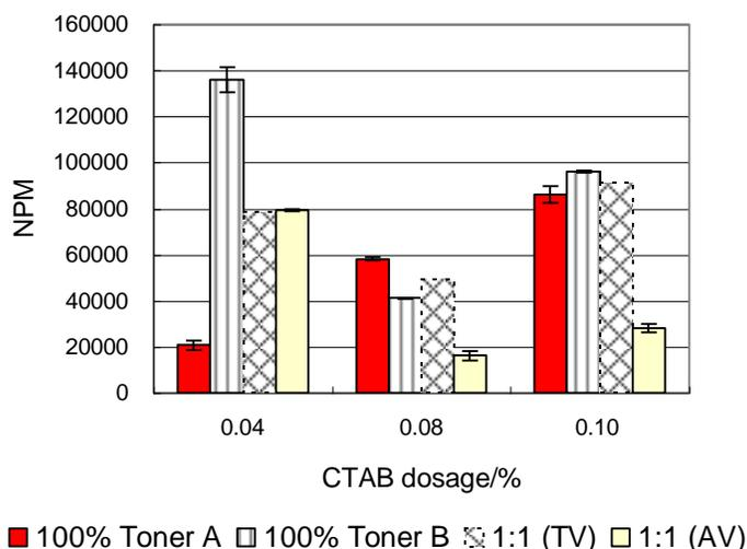
**Fig. 7.** Effect of CTAB on NPM after agglomeration of two toners mixed by the ratio of 1:1 with 2.0% 1-octadecanol
