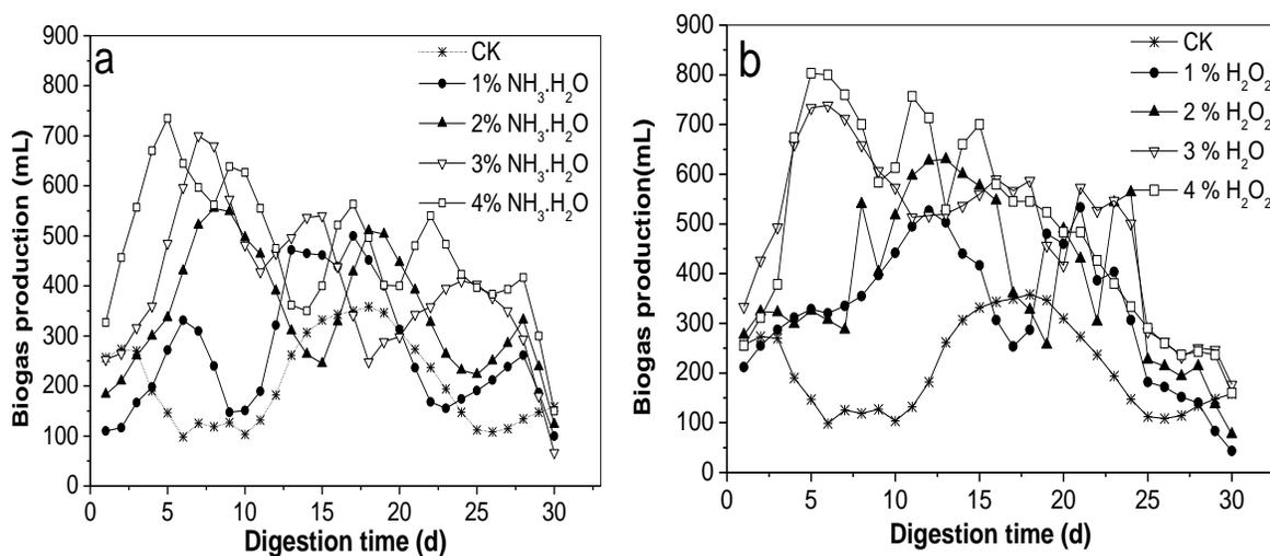
**Fig. 2.** Daily biogas production for each pretreatment. (a)  $\text{NH}_3 \cdot \text{H}_2\text{O}$  and (b)  $\text{H}_2\text{O}_2$  pretreatments
