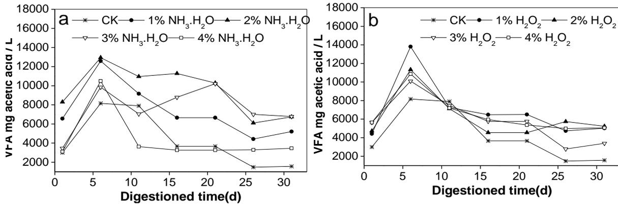
Fig. 6. VFA changes for each pretreatment. (a)  $\text{NH}_3\cdot\text{H}_2\text{O}$  and (b)  $\text{H}_2\text{O}_2$  pretreatment. CK: Rice straw without pretreatment
