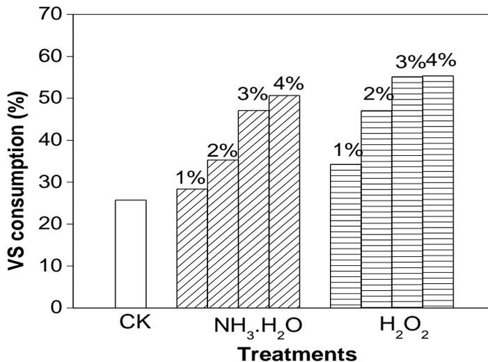
Fig. 4. Volatile solids (VS) consumption of each pretreatment. CK: Rice straw without pretreatment
