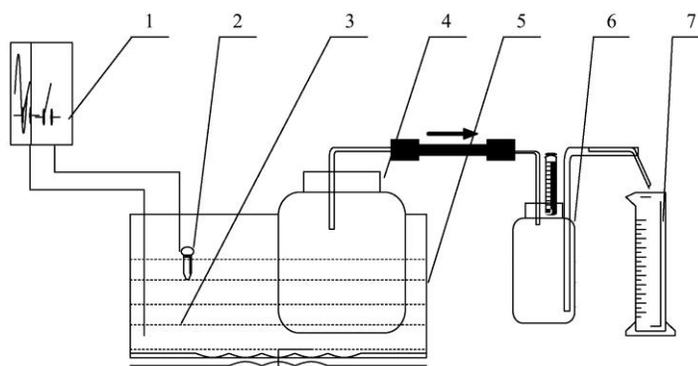
**Fig. 1.** Controllable and constant-temperature anaerobic fermentation device: 1. Relay; 2. Temperature controller; 3. Heater; 4. Anaerobic digester; 5. Trough at constant temperature; 6. Receiver; 7. Measuring cylinder
