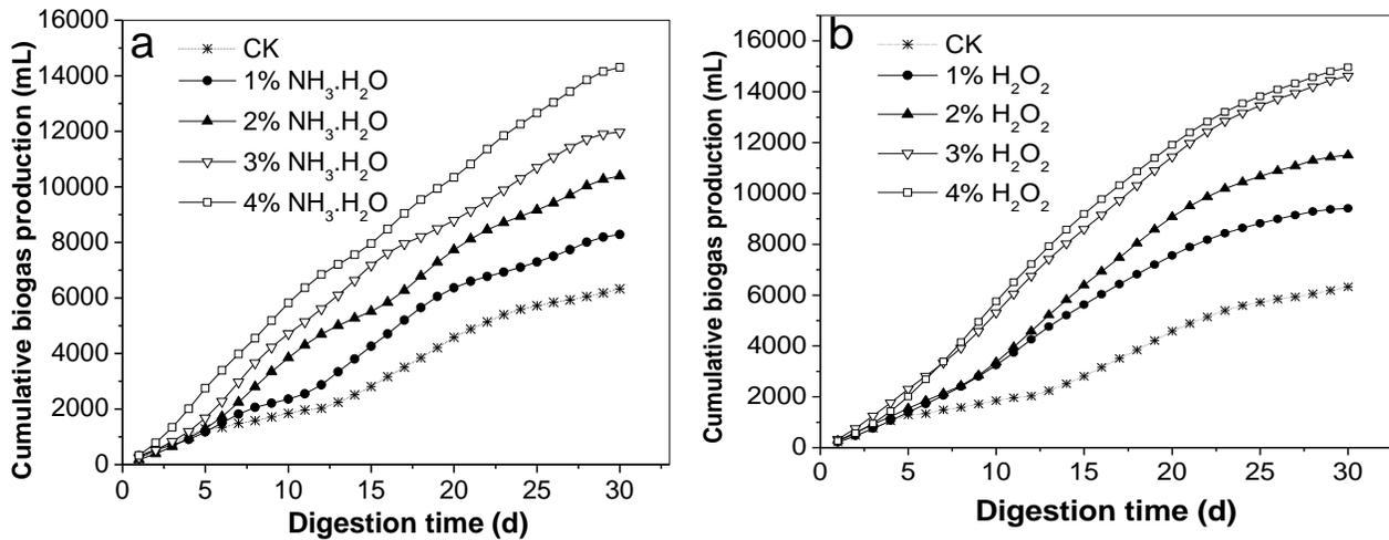
Fig. 3. Cumulative biogas production of each pretreatment. (a)  $\text{NH}_3 \cdot \text{H}_2\text{O}$  and (b)  $\text{H}_2\text{O}_2$  pretreatments. CK: Rice straw without pretreatment
