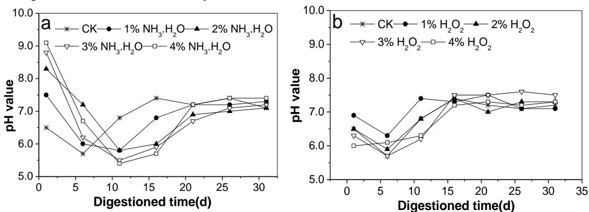
**Fig. 5.** Variations in pH value for each pretreatment. (a)  $\text{NH}_3\cdot\text{H}_2\text{O}$  and (b)  $\text{H}_2\text{O}_2$  pretreatments. CK: Rice straw without pretreatment
