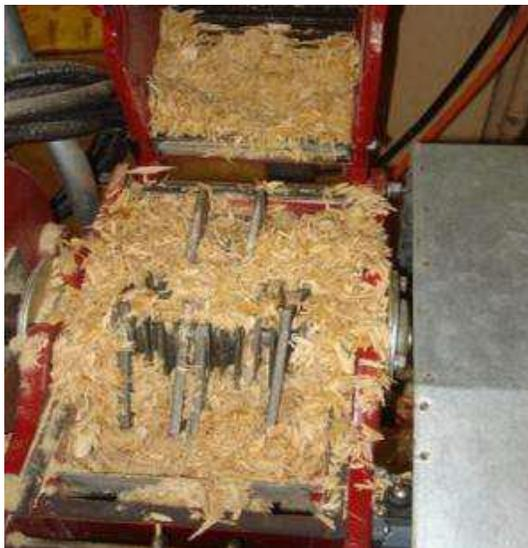
**Fig. 5.** Overloading and bundling caused by high moisture chips entering a hammermill chamber (Arrieche 2010)
