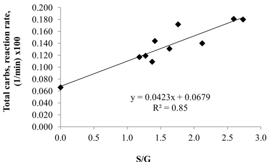
Fig. 6. Carbohydrates degradation ratio as a function of S/G ratio
