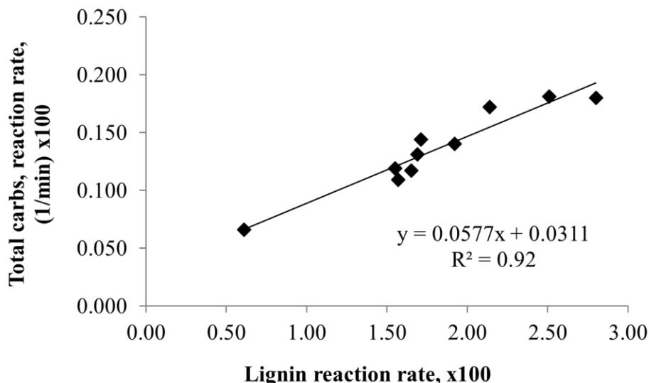
Fig. 7. Delignification ratio as a function of carbohydrates degradation
