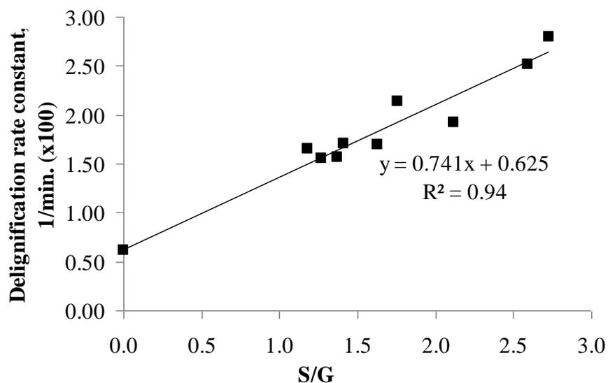
Fig. 5. Delignification ratio as a function of S/G ratio
