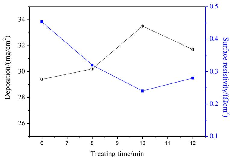
**Fig. 2.** The effects of NaBH<sub>4</sub> treating time on the deposition and surface resistivity of the plated veneers (pH of the plating solution 12.25, plating time 30 min)
