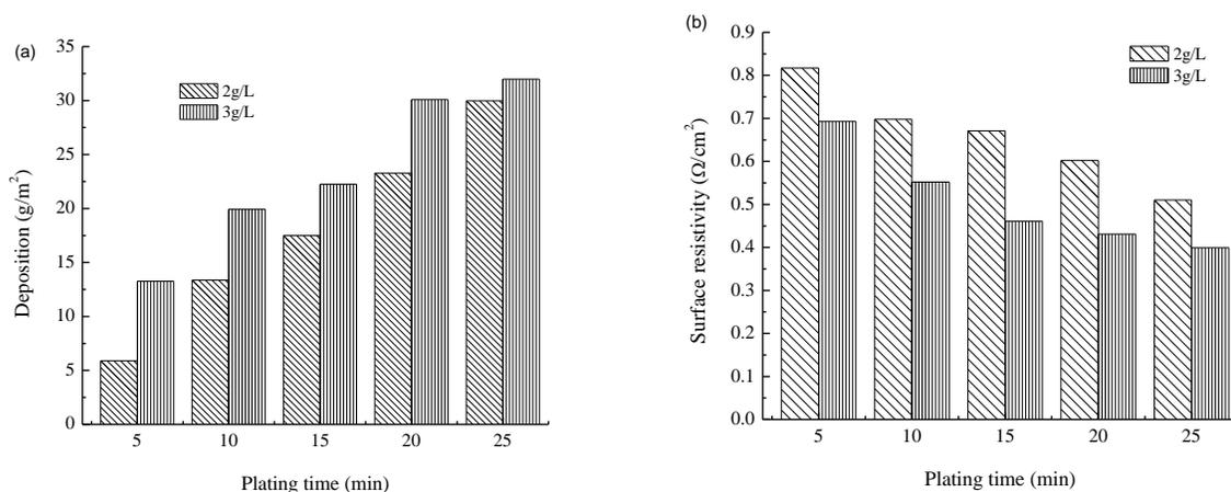
**Fig. 4.** The effects of plating time on (a) the deposition and (b) surface resistivity of the plated veneers
