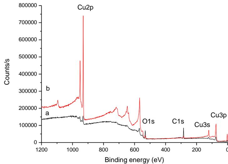
**Fig. 8.** XPS spectrum of copper coating on *Fraxinus mandshurica* veneer (a) surface and (b) etched
