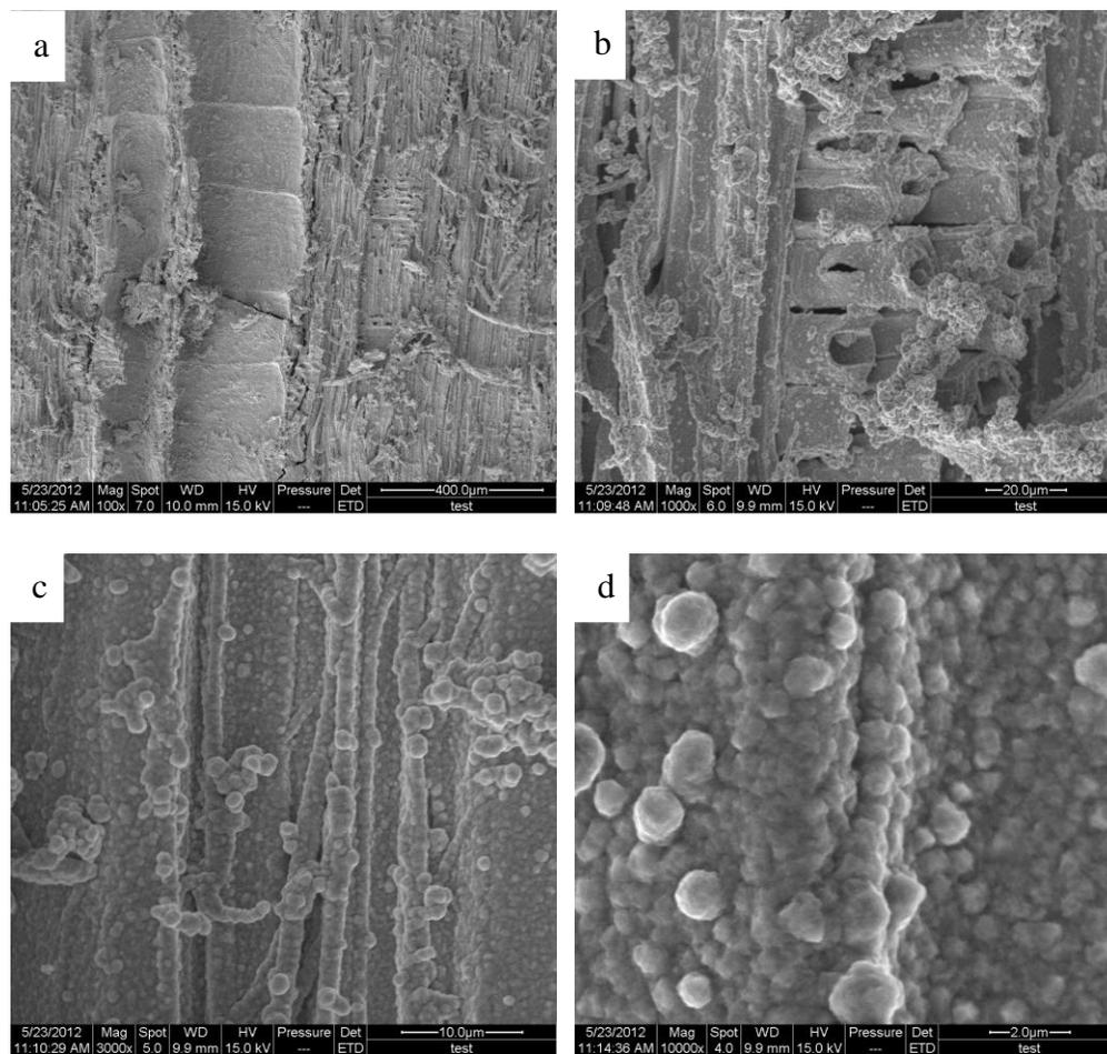
**Fig. 5.** Morphology of plated *Fraxinus mandshurica* veneers (a) overall surface 100x; (b) xylem ray; (c) inner wall of vessel; (d) pits with high magnification
