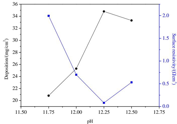
**Fig. 3.** The relationship between the pH of the plating solution and the deposition and surface resistivity of the plated veneers
