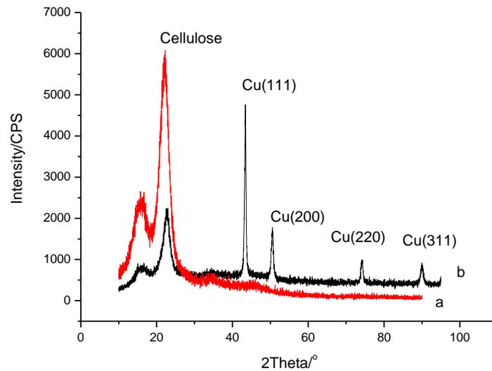
**Fig. 10.** XRD patterns of *Fraxinus mandshurica* veneer (a) before and (b) after being plated with copper coating
