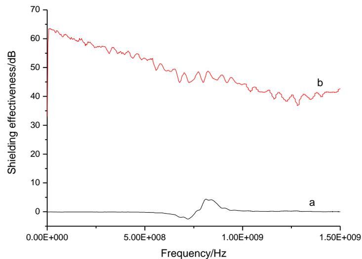
**Fig. 11.** Electromagnetic shielding effectiveness of *Fraxinus mandshurica* veneers (a) before and (b) after copper plating
