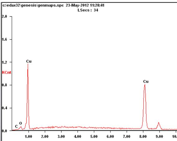
Fig. 7. EDS spectrum of the copper-plated veneer
