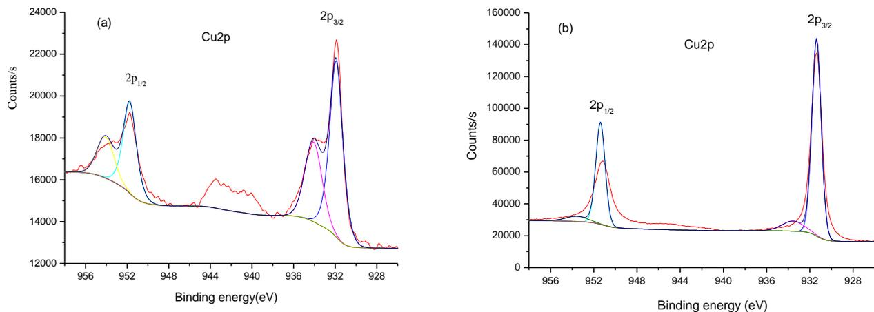
**Fig. 9.** High-resolution XPS spectra of Cu2p of the coating (a) surface and (b) etched
