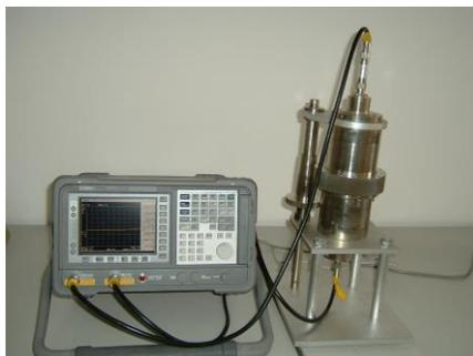
**Fig. 1.** The instrument for measuring electromagnetic shielding effectiveness
