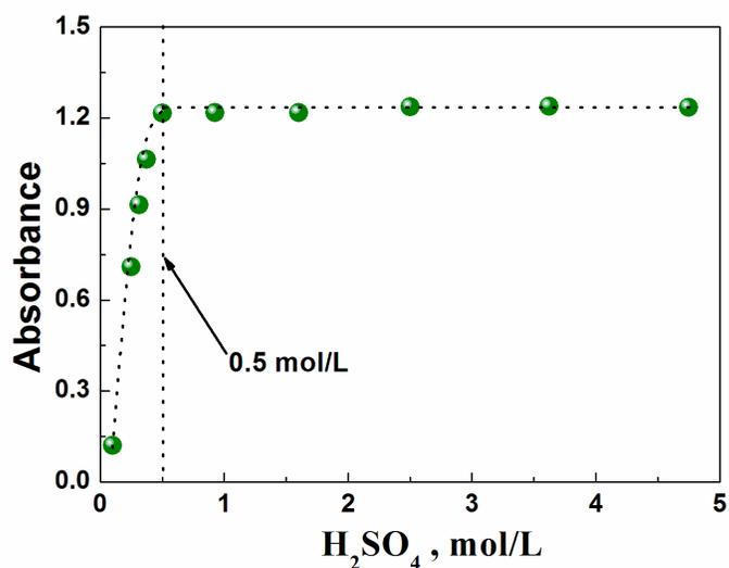
Fig. 3. Effect of H<sub>2</sub>SO<sub>4</sub> concentration
