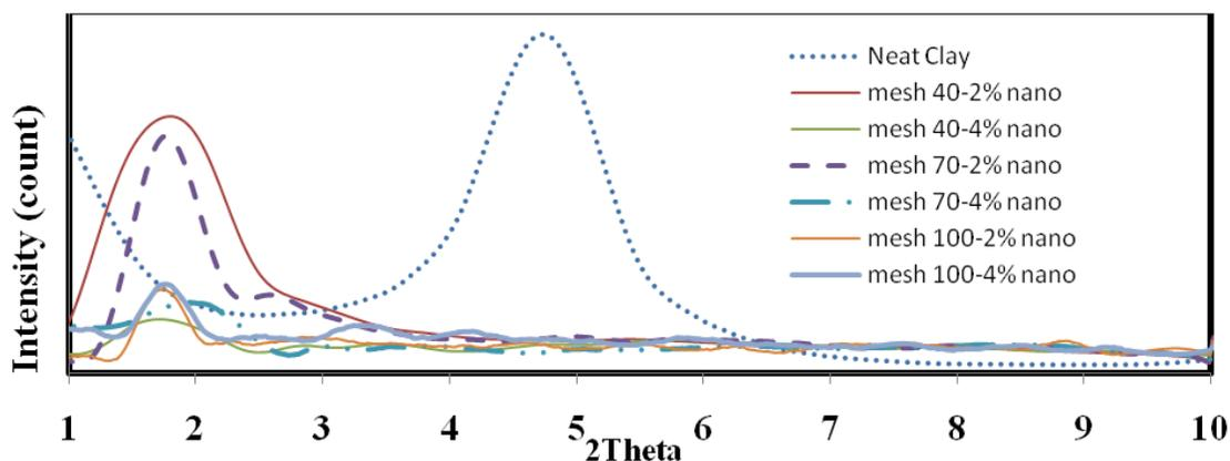
Fig. 6. XRD patterns of nanoclay content at  $2\theta = 1$  to  $10^\circ$
