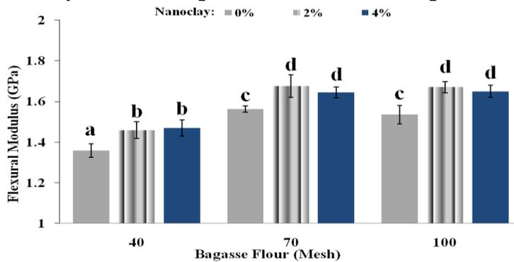
Fig. 4. Effect on nanoclay and size of bagasse flour on flexural modulus of nanocomposite
