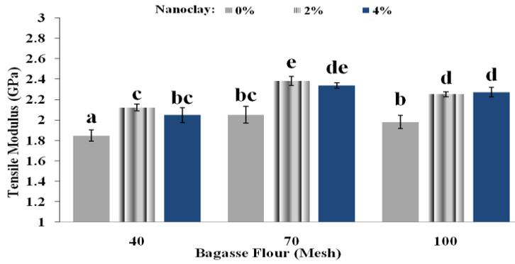
Fig. 2. Effect on nanoclay and size of bagasse flour on tensile modulus of nanocomposite
