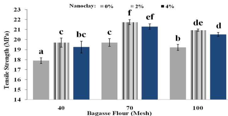
**Fig. 1.** Effect on nanoclay and size of bagasse flour on tensile strength of nanocomposite
