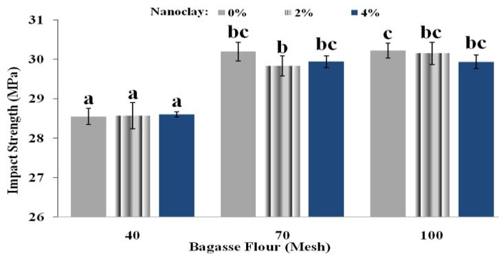
Fig. 5. Effect on nanoclay and size of bagasse flour on impact strength of nanocomposite
