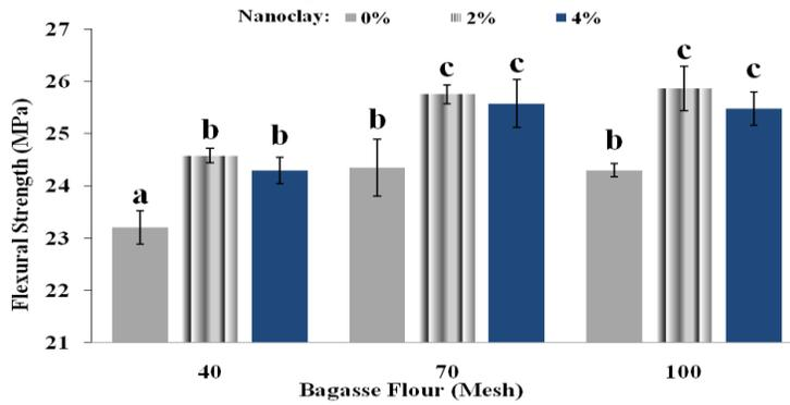
Fig. 3. Effect on nanoclay and size of bagasse flour on flexural strength of nanocomposite
