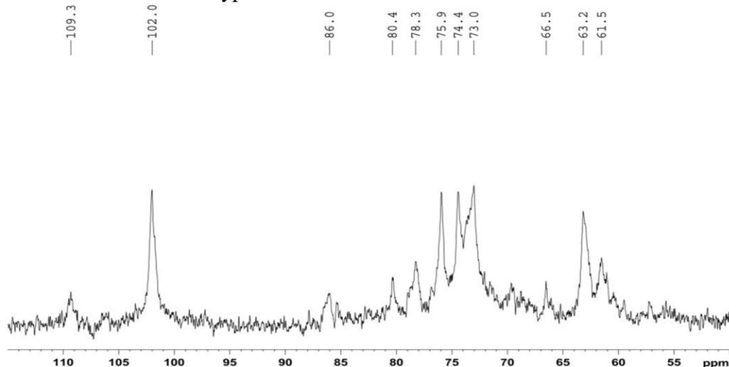
**Fig. 5.**  $^{13}\text{C}$ -NMR spectrum of hemicellulosic fraction  $\text{H}_6$  isolated with 60% ethanol containing 0.25 M NaOH at 75 °C for 3 h
