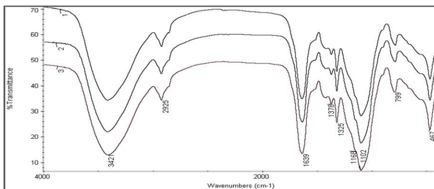
**Fig. 2.** FT-IR spectra of rice straw hemicellulosic fractions isolated with 60% methanol (spectrum 1), 60% ethanol (spectrum 2), and 60% n-propanol (spectrum 3) at 75 °C for 3 h
