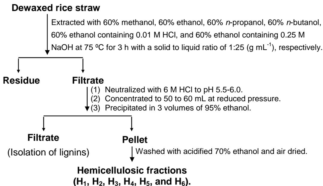
Fig. 1. Scheme for isolation of hemicelluloses from rice straw
