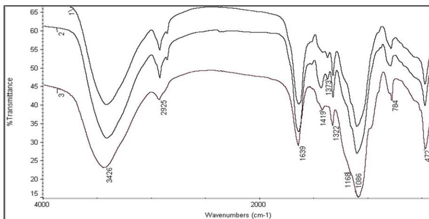
**Fig. 3.** FT-IR spectra of rice straw hemicellulosic fractions isolated with 60% n-butanol (spectrum 1), 60% ethanol containing 0.01 M HCl (spectrum 2), and 60% ethanol containing 0.25 M NaOH (spectrum 3) at 75 °C for 3 h
