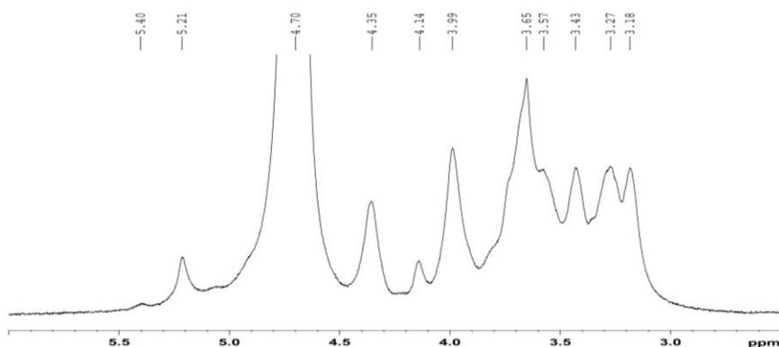
**Fig. 4.** <sup>1</sup>H-NMR spectrum of hemicellulosic fraction H<sub>6</sub> isolated with 60% ethanol containing 0.25 M NaOH at 75 °C for 3 h
