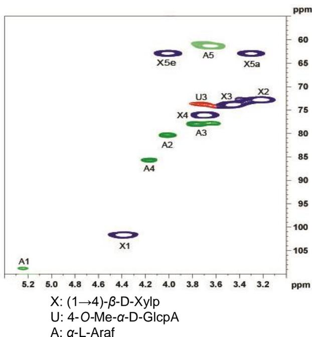
**Fig. 6.** 2D-HSQC spectrum of hemicellulosic fraction H<sub>6</sub> isolated with 60% ethanol containing 0.25 M NaOH at 75 °C for 3 h
