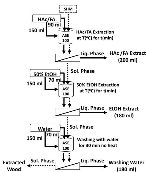
**Fig. 2.** Two-stage fractionation process of SHM chips with 50% EtOH following acid-reinforced autohydrolysis
