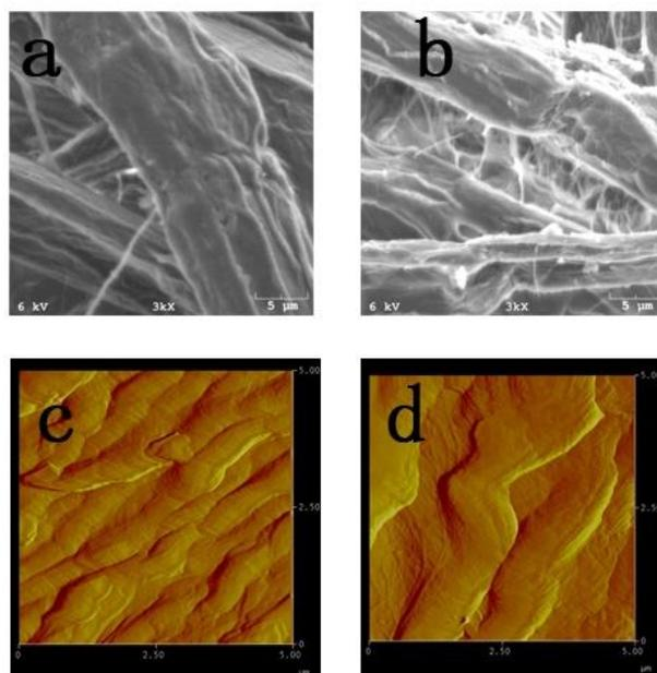
**Fig. 4.** SEM micrograph of bamboo fiberboard made from bamboo fibers (a) and made from bamboo fibers treated with 1.5% CGG (b), and AFM ultra-microstructure analysis of fiber treated with CGG with 1.5% CGG (c) and untreated bamboo fiber (d)
