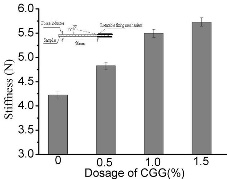
Fig. 2. Effect of CGG on stiffness properties of bamboo fiber fiberboard
