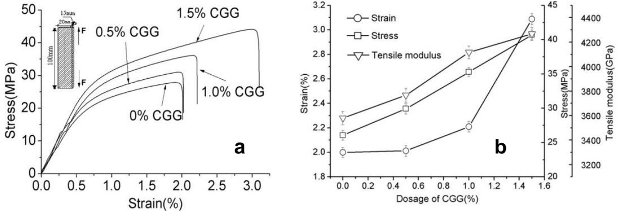
Fig. 1. Tensile stress-strain curves (a) and the effect of CGG on the tensile property (b) of bamboo fiberboard
