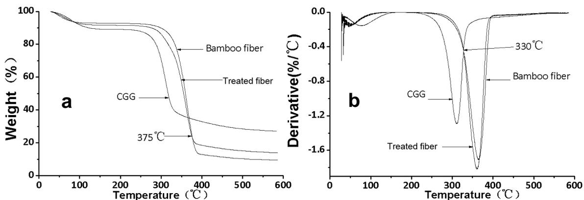
**Fig. 3.** TGA (a) and DTG (b) curves of untreated and treated bamboo fiber
