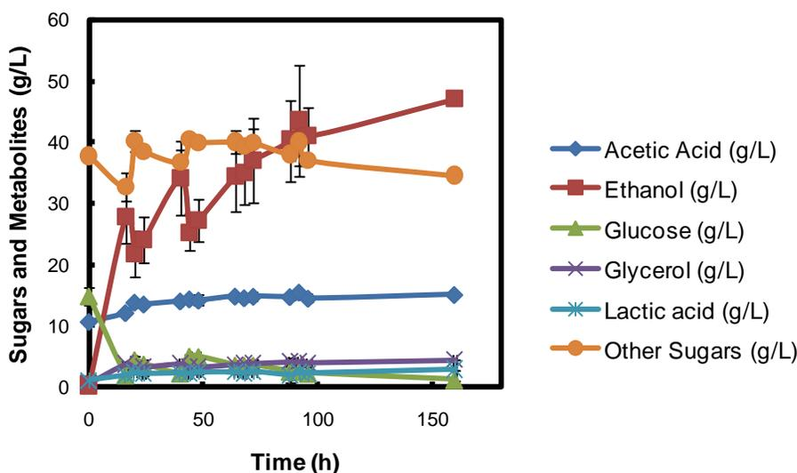
**Fig. 2.** Sugar and metabolite concentrations during SSF with 12% SS
