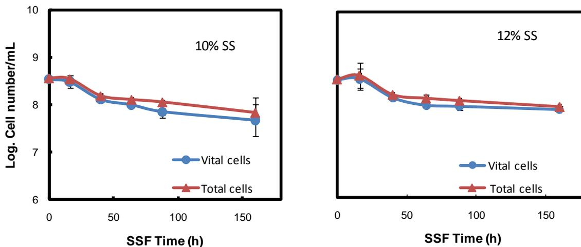
**Fig. 5.** Logarithm values of yeast cell number/mL versus time (h) during SSF with 10% and 12% suspended solids
