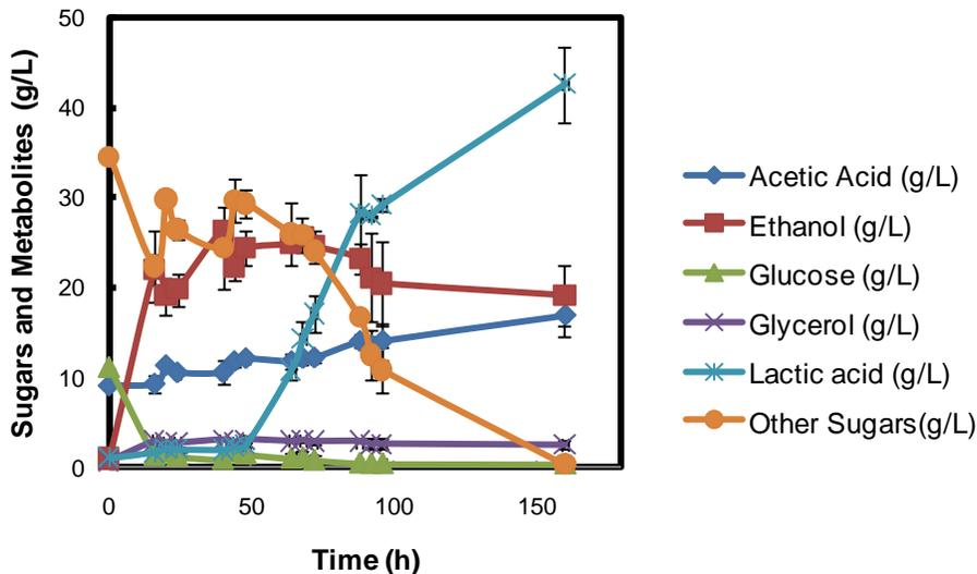
Fig. 3. Sugar and metabolite concentrations during SSF with 10% SS
