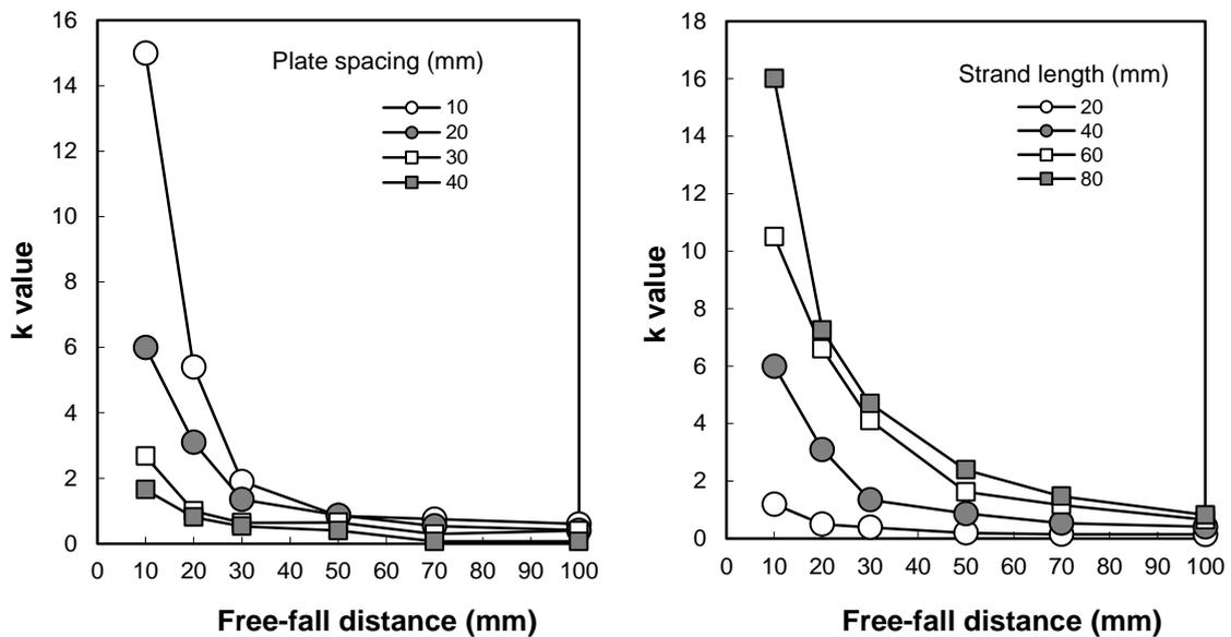
**Fig. 3.** The effect of free-fall distances on  $k$  values at various plate spacings (left) and strand lengths (right), using 40 mm strands. (The  $k$  value in the figure was obtained by least square method.)
