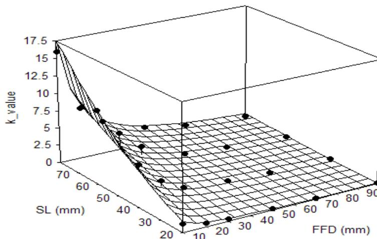
**Fig. 4.** The sample concentration parameter ( $k$  value) of the von Mises distribution as a function of strand length and free-fall distances at a plate spacing of 20 mm (Equation 2)
