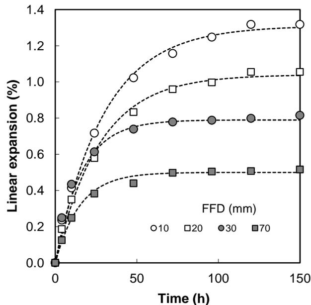
**Fig. 5.** Linear expansion (LE) behaviors in the perpendicular direction for bamboo OSB at various FFDs
