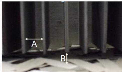
**Fig. 1.** Plate spacing (A) and free fall distance (B) of a manual-aligning device (redrawn from Sumardi *et al.* 2008)
