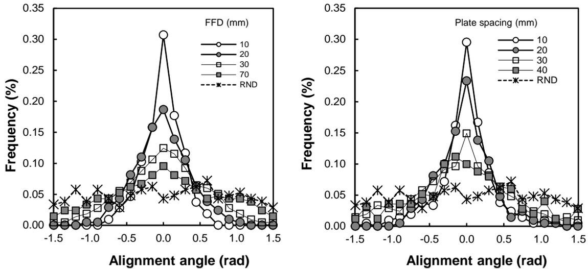
**Fig. 2.** The plotted data points of strand alignment angle at various free-fall distances (left) and plate spacings (right) using strands of 40 mm length
