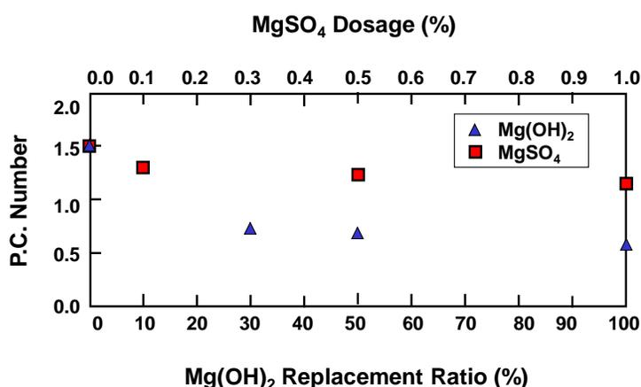
Fig. 2. The effect of the  $\text{Mg}(\text{OH})_2$  replacement ratio and  $\text{MgSO}_4$  dosage on the P.C. number
