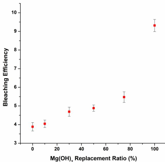
**Fig. 1.** The effect of the  $\text{Mg}(\text{OH})_2$  replacement ratio on bleaching efficiency (Error bars: one standard deviation)
