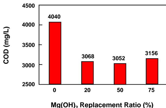
Fig. 3. The effect of the  $\text{Mg}(\text{OH})_2$  replacement ratio on COD
