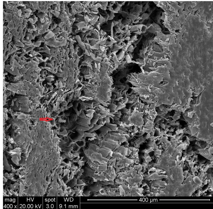
**Fig. 5.** Red cedar sample exposed to a temperature of 160 °C for 7 h
