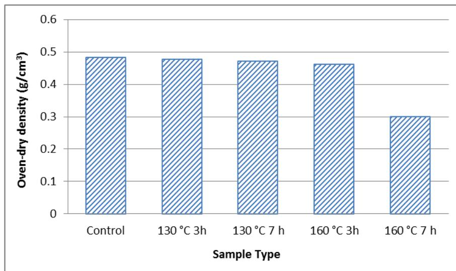
**Fig. 1.** Oven-dry density values of the specimens
