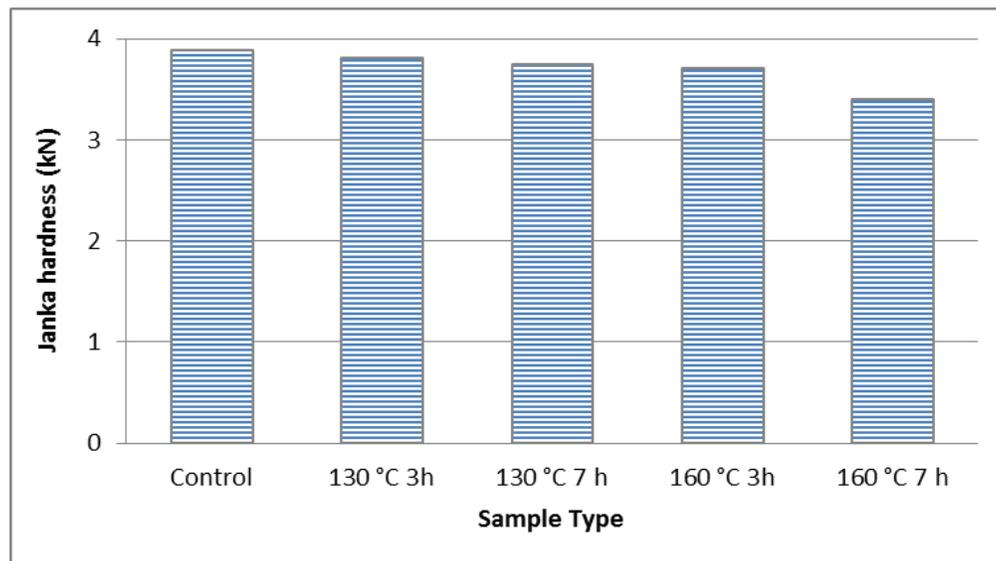
Fig. 4. Janka hardness values of the specimens
