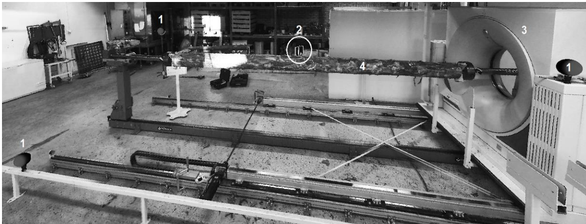
Fig. 1. Setup for data acquisition. (1) Reference points; (2) 3D phase-shift laser scanner; (3) Computer tomography scanner and (4) the Scots pine log.
