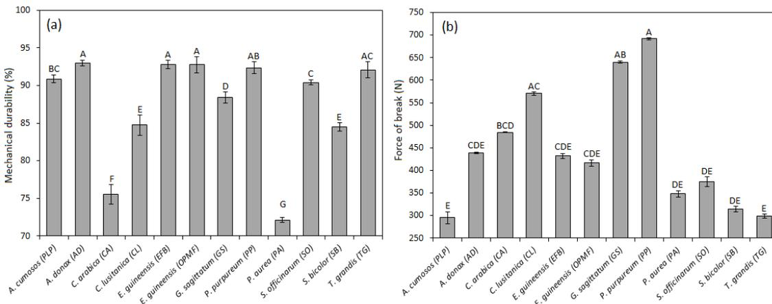
**Fig. 1.** (a) Mechanical durability and (b) force at break of 12 pellet crops in Costa Rica. Legend: Different letters for each crop represent statistical difference between crops (significances at 95%)
