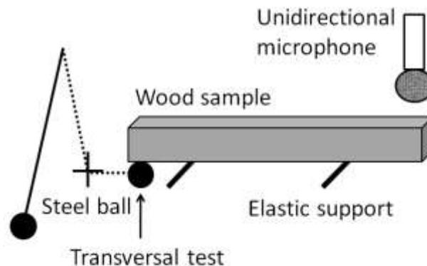
Fig. 1. Schematic view of the beam under flexural vibration
