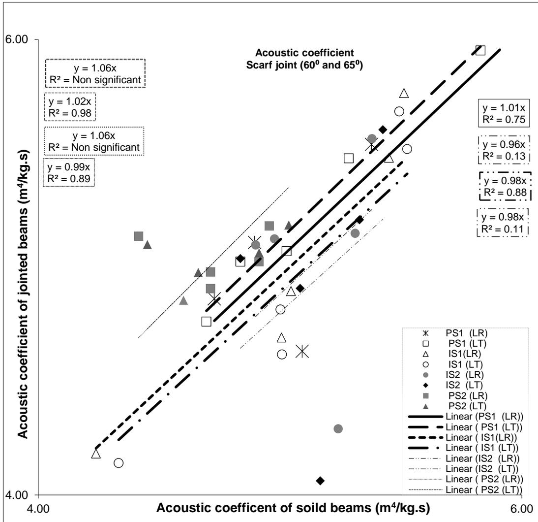
**Fig. 3.** The acoustic coefficient (m<sup>4</sup>kg.s) obtained from *LR* and *LT* flexural vibration for 60° and 65° scarf jointed beams *versus* reference solid beams
