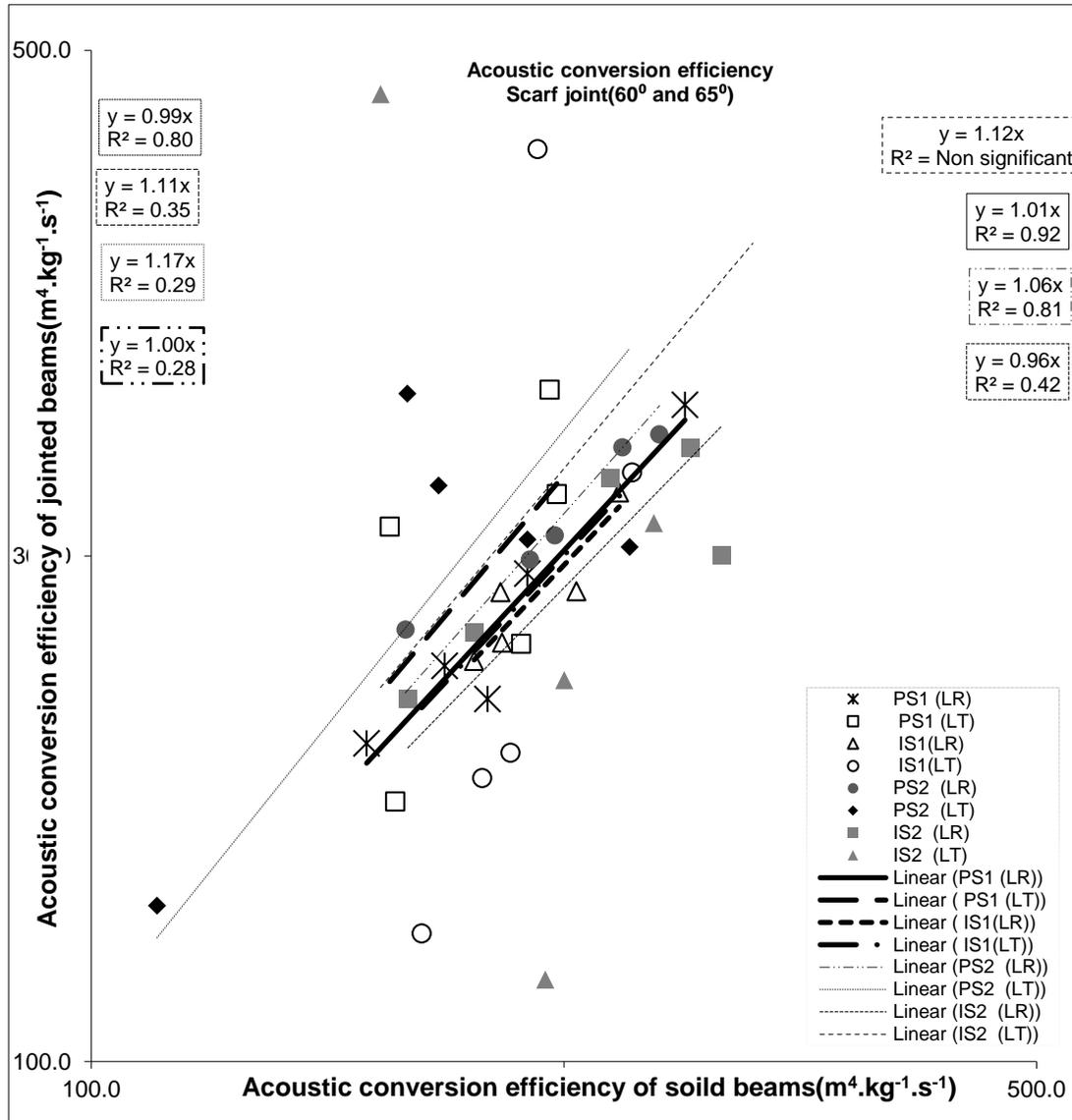
**Fig. 4.** The acoustic conversion efficiency obtained from LR and LT flexural vibration for 60° and 65° scarf jointed beams versus reference solid beams
