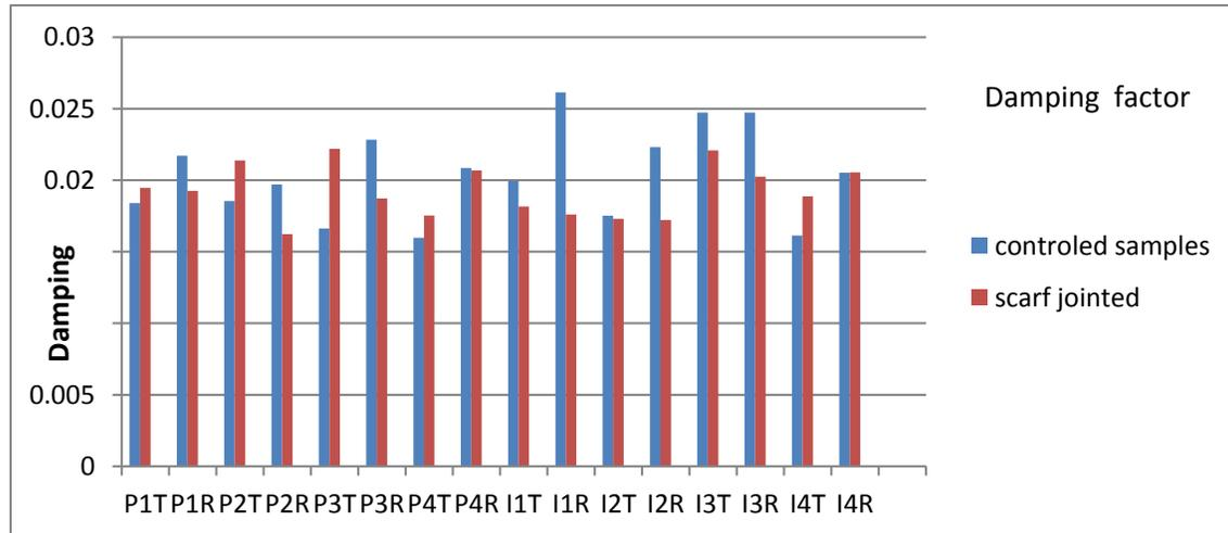
**Fig. 7.** Damping comparison obtained from *LR* and *LT* flexural vibration for scarf jointed beams versus reference solid beams. (Adhesive used: I=Isocyanate, P=Polyvinyl acetate, Angle: 1=60°, 2=65°, 3=70°, and 4=75°)
