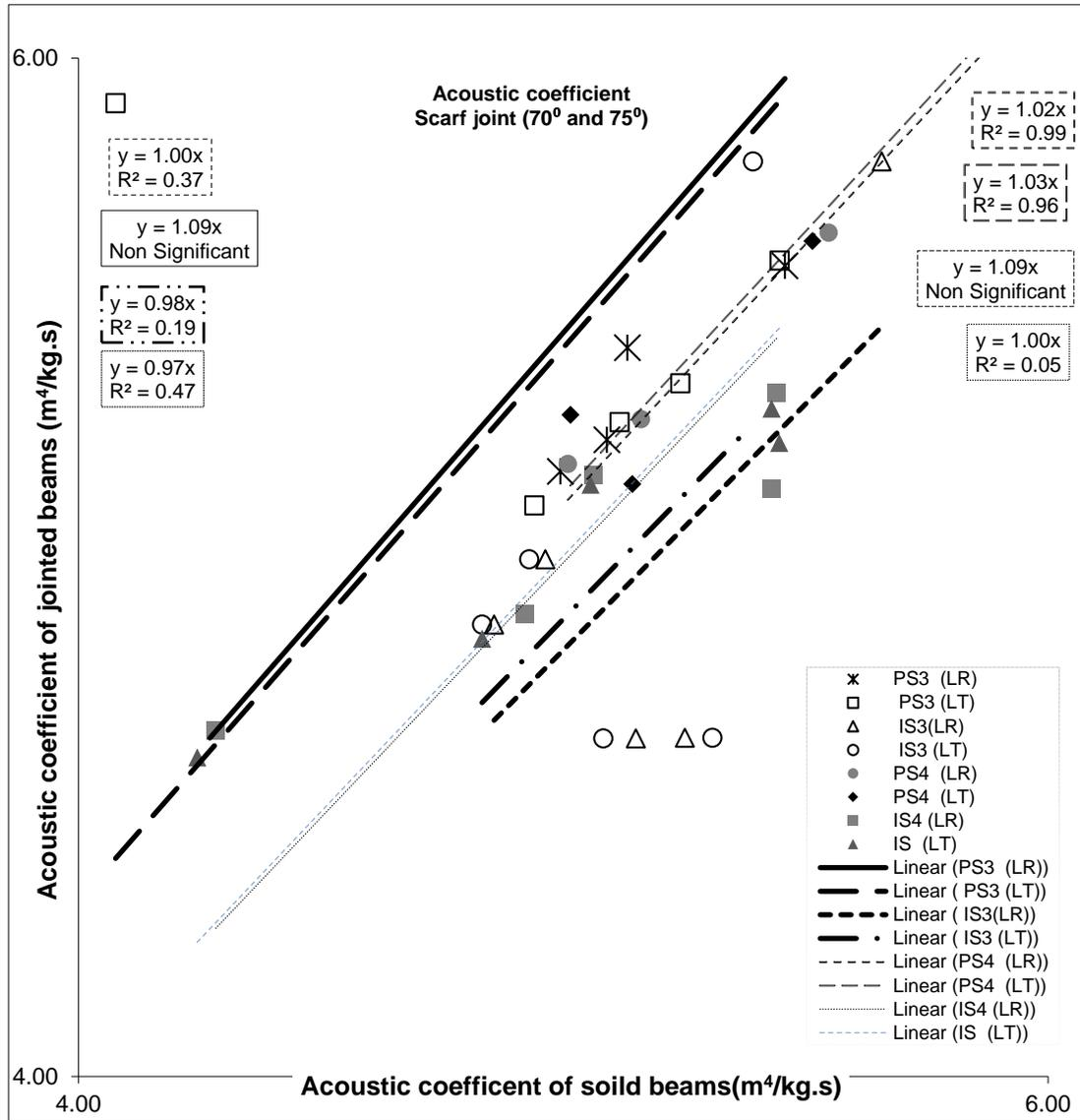
**Fig. 5.** The acoustic coefficient (m<sup>4</sup>/kg.s) obtained from *LR* and *LT* flexural vibration for 70° and 75 ° scarf jointed beams *versus* reference solid beams
