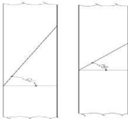
**Fig. 2.** The 60° and 75° scarves as an example of beams jointed with different scarf angles
