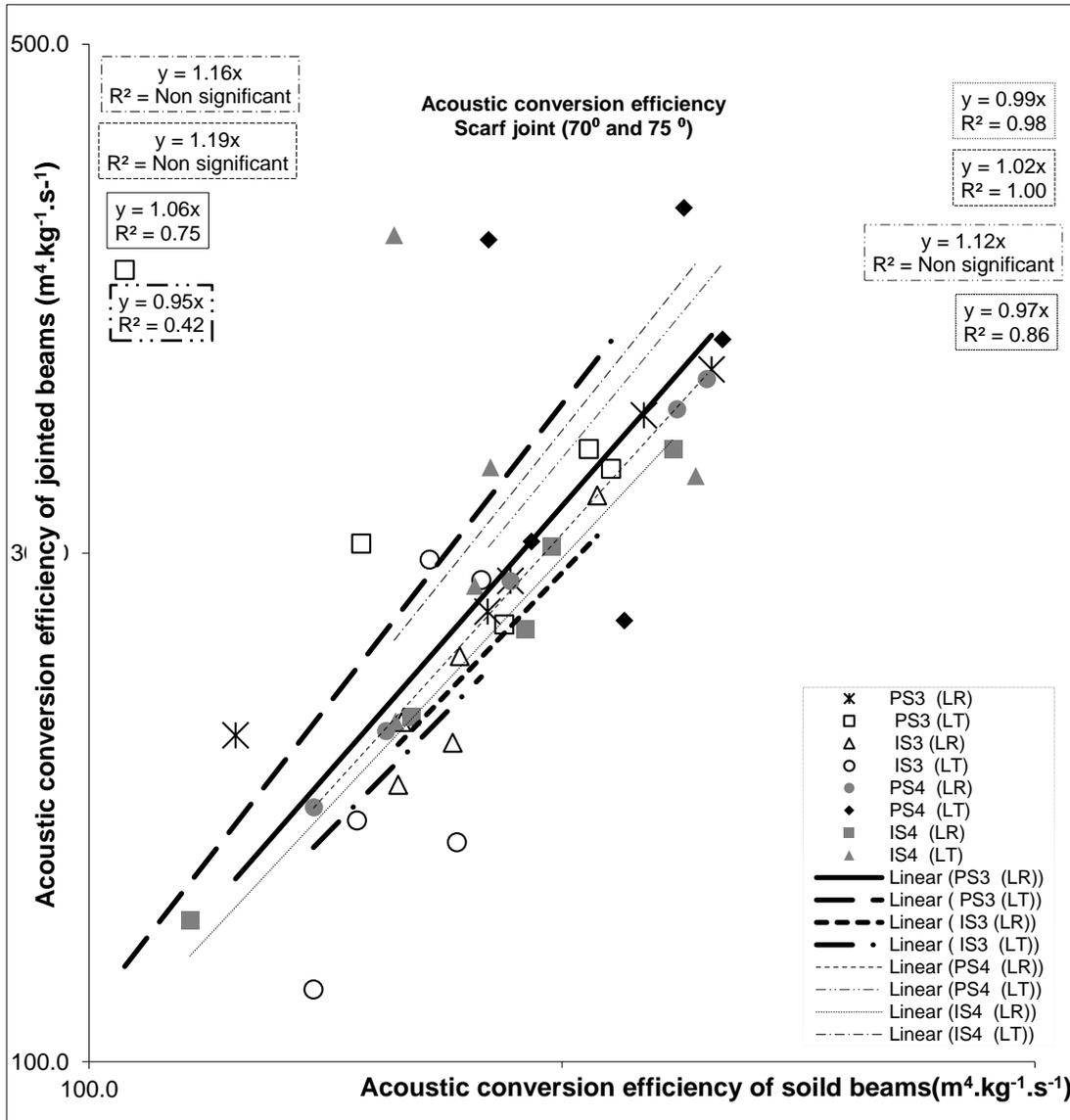
**Fig. 6.** The acoustic conversion efficiency obtained from LR and LT flexural vibration for 70° and 75° scarf jointed beams versus reference solid beams
