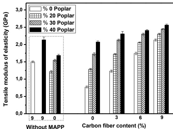
Fig. 4. Effect of carbon fiber content on tensile modulus of elasticity of PP and composites
