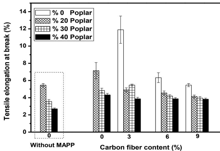
Fig. 5. Effect of carbon fiber content on tensile elongation at break of PP and composites
