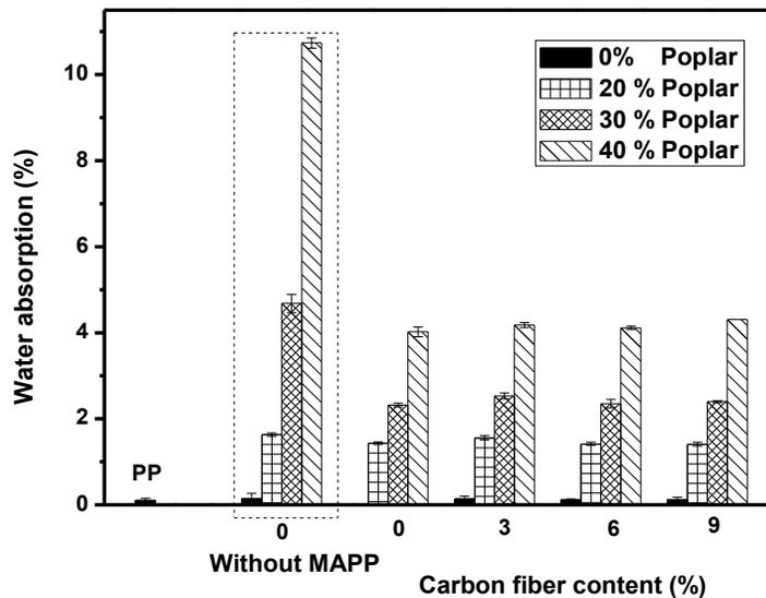
Fig. 2. Effect of carbon fiber content and MAPP on water absorption of PP and composites after 125 days of water immersion
