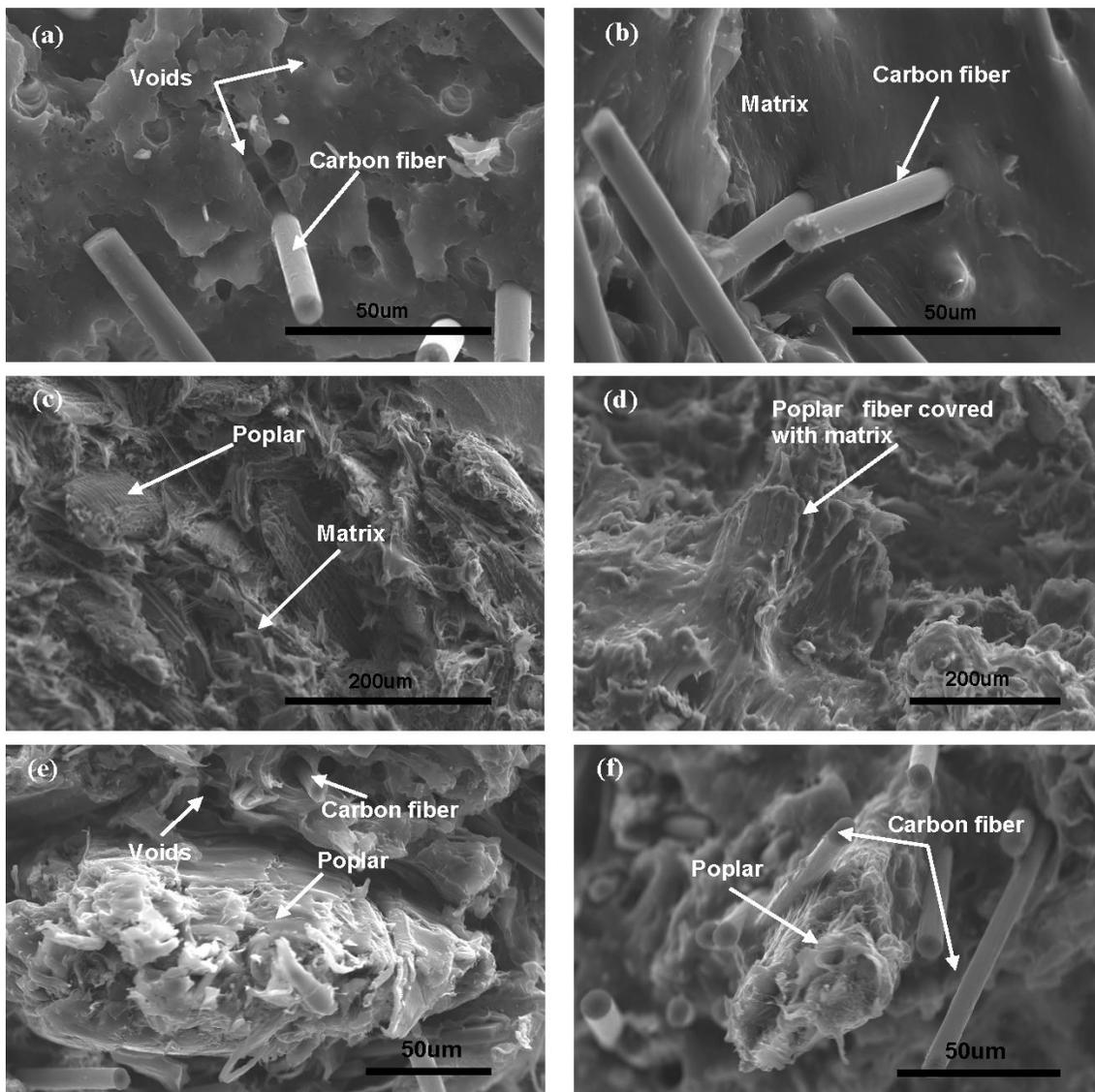
**Fig. 9.** SEM micrographs of tensile fractured surfaces of composites: (a) PP91/CF9, (b) PP88/CF9/MAPP3, (c) POP40/PP60, (d) POP40/PP57/MAPP3, (e) POP40/PP51/CF9, and (f) POP40/PP48/CF9/MAPP3. Note the scale indication (black) at the lower right of each image.
