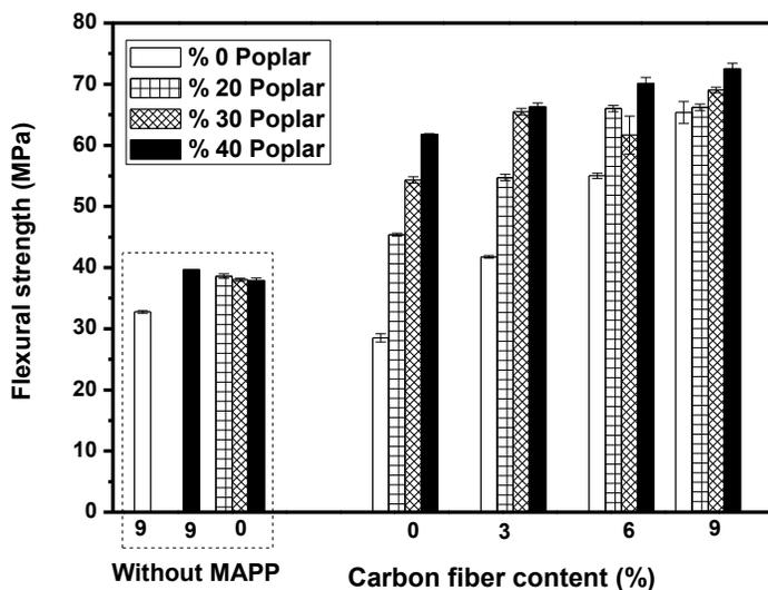
Fig. 7. Effect of carbon fiber content on flexural strength of PP and composites
