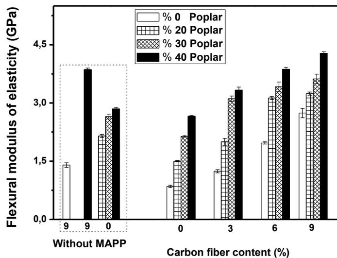
Fig. 6. Effect of carbon fiber content on flexural modulus of elasticity of PP and composites
