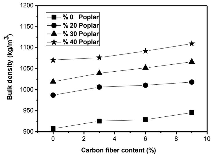
Fig. 1. Effect of carbon fiber content on the bulk density of PP and composites
