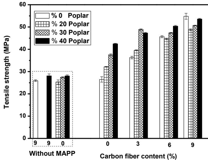
Fig. 3. Effect of carbon fiber content on tensile strength of PP and composites
