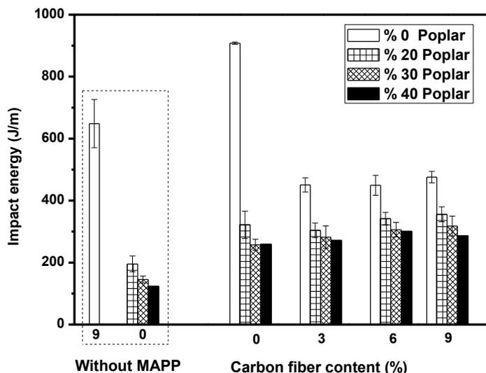
Fig. 8. Effect of carbon fiber content on impact energy of PP and composites
