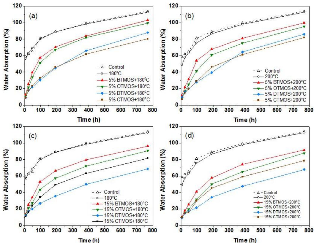
**Fig. 4.** Water absorption of wood not treated, thermally-treated, or treated with (a) 5% AAS + 180 °C, (b) 5% AAS + 200 °C, (c) 15% AAS + 180 °C, and (d) 15% AAS + 200 °C
