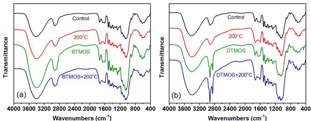
**Fig. 9.** FTIR spectra of BTMOS-thermally modified wood (a); DTMOS-thermally modified wood (b)
