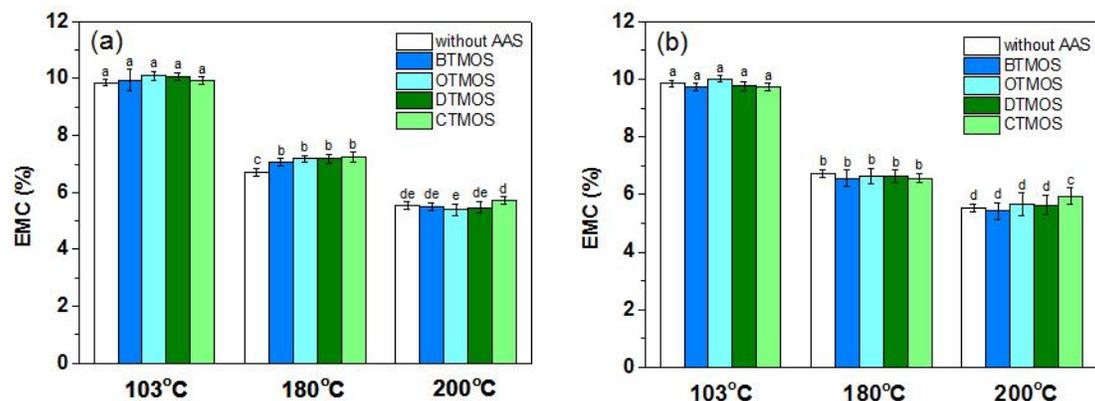
**Fig. 6.** The EMC of 5% (a) and 15% (b) AAS-modified and unmodified wood. Bars accompanied by different letters (a, b, c, d, and e) are significantly different at  $p < 0.05$  (Duncan test).
