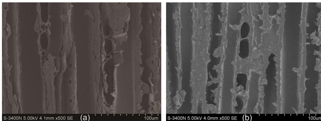
**Fig. 10.** SEM images of tangential sections from 200 °C thermally modified (a) and DTMOS-200 °C thermally modified wood (b)
