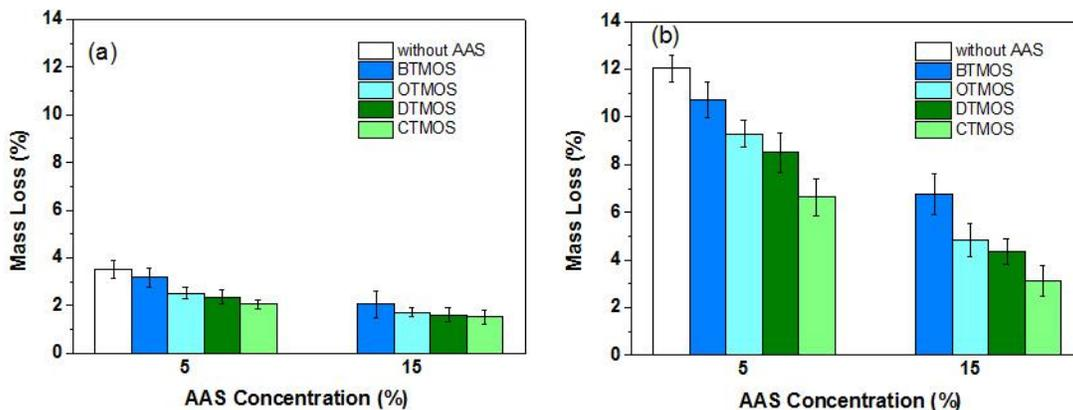
Fig. 3. MLs of wood samples thermally modified at 180°C (a), and 200°C (b)
