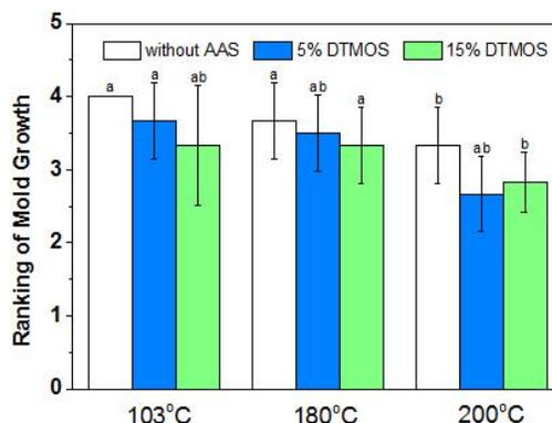
Fig. 8. Ranking of mold growth on modified and unmodified wood
