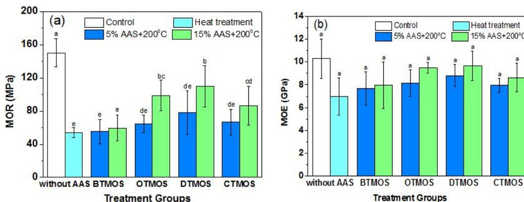
**Fig. 7.** The MOR (a) and MOE (b) of treated wood samples. Bars accompanied by different letters (a, b, c, d, and e) are significantly different at  $p < 0.05$  (Duncan test).
