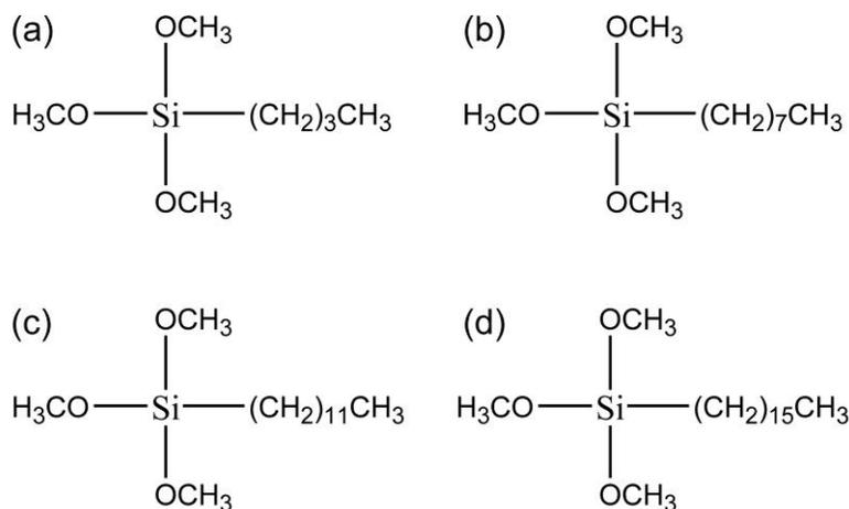
**Fig. 1.** The chemical structures of BTMOS (a), OTMOS (b), DTMOS (c), and CTMOS (d)
