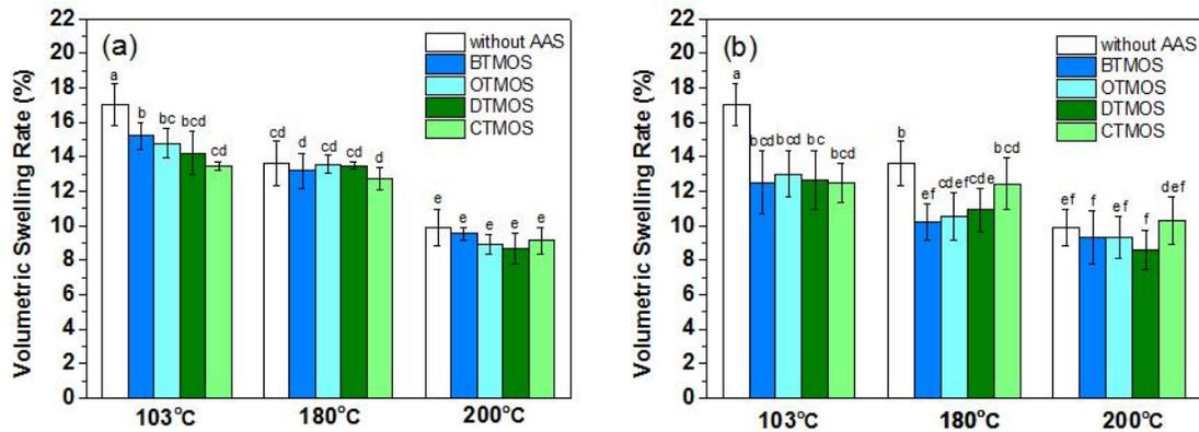
**Fig. 5.** Volumetric swelling rates of the wood treated with 5% (a) and 15% (b) AAS. Bars accompanied by different letters (a, b, c, d, e, and f) are significantly different at  $p < 0.05$  (Duncan test).
