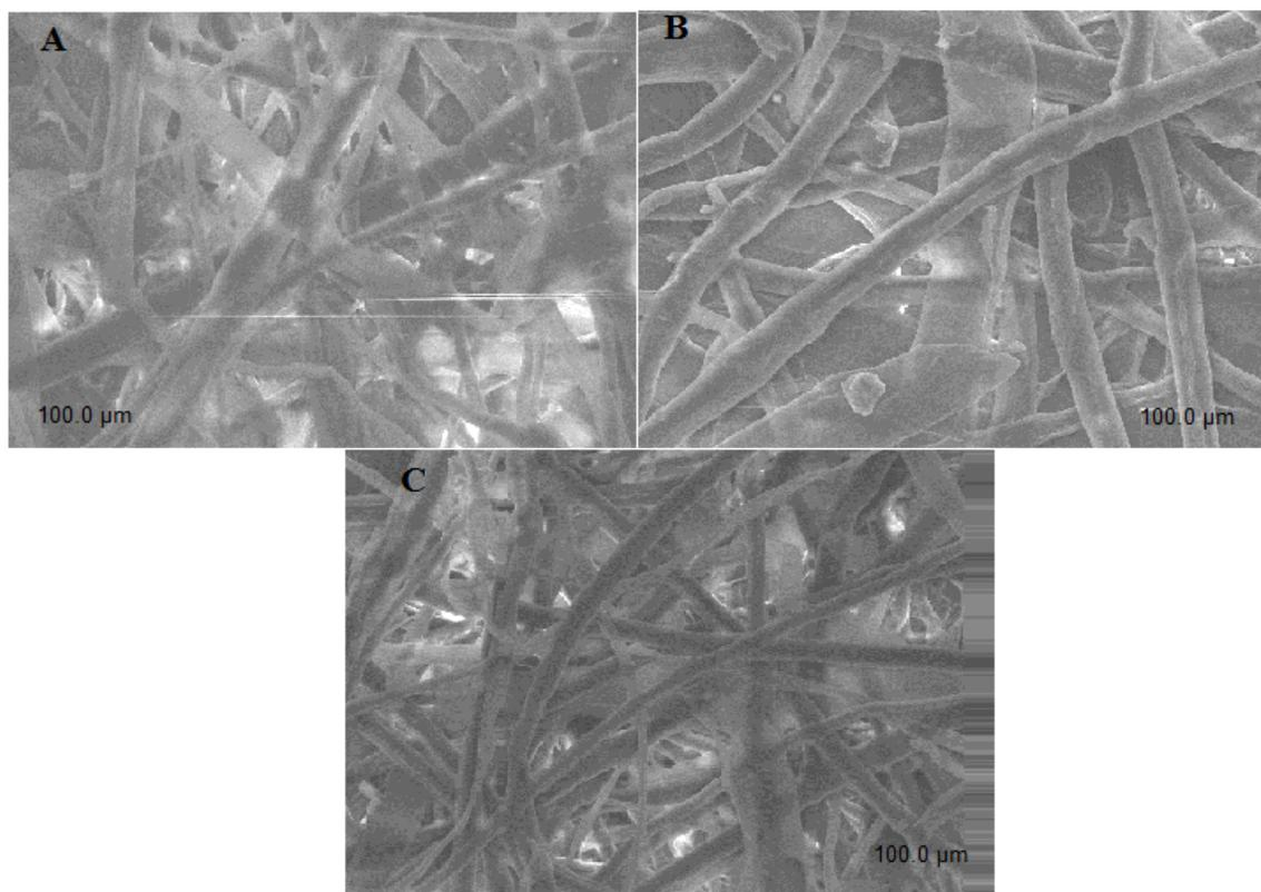
**Fig. 3.** Scanning electron microscope images of millet stalks (A), date palm leaves (B), and 50% blend (C)
