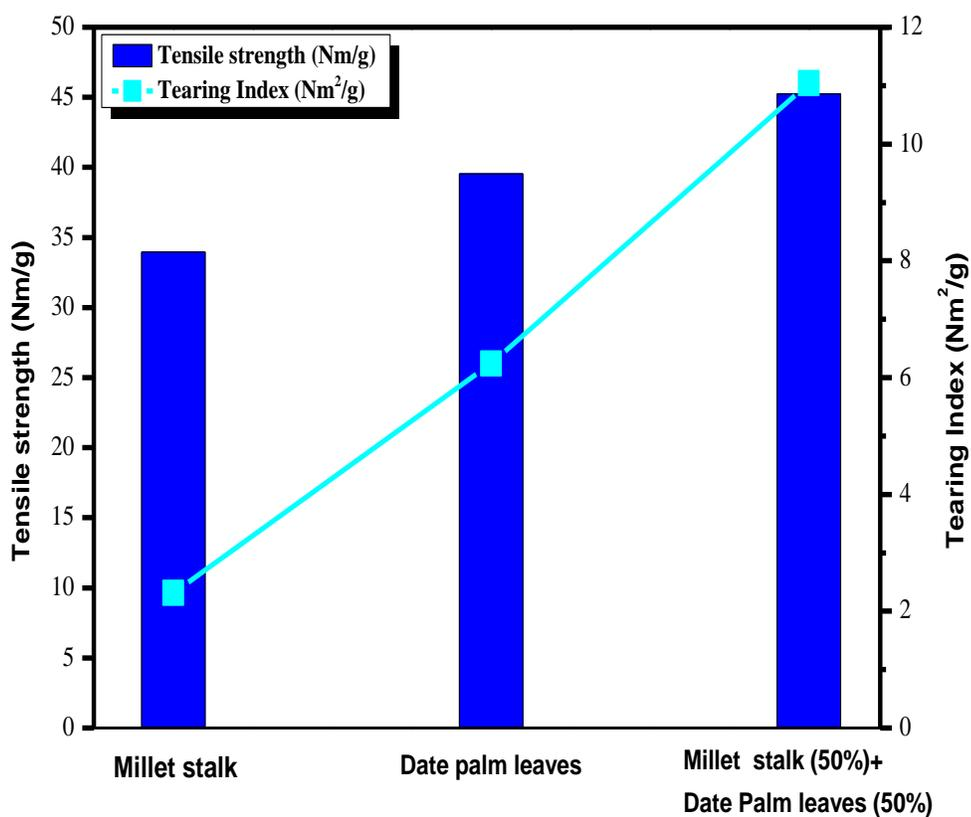
**Fig. 2.** Tensile strength and tearing index of the materials
