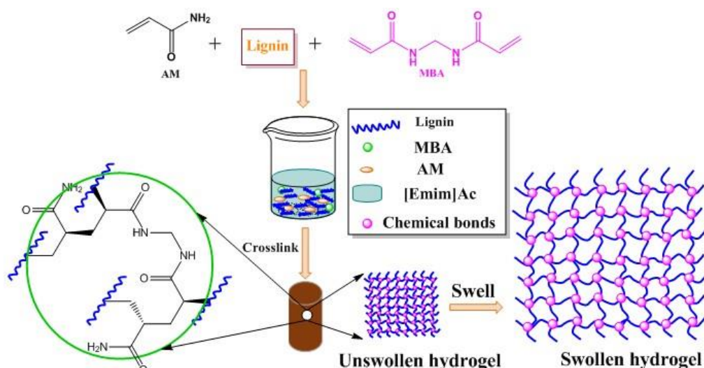
Fig. 2. Schematic diagram of the green synthesis of LCH
