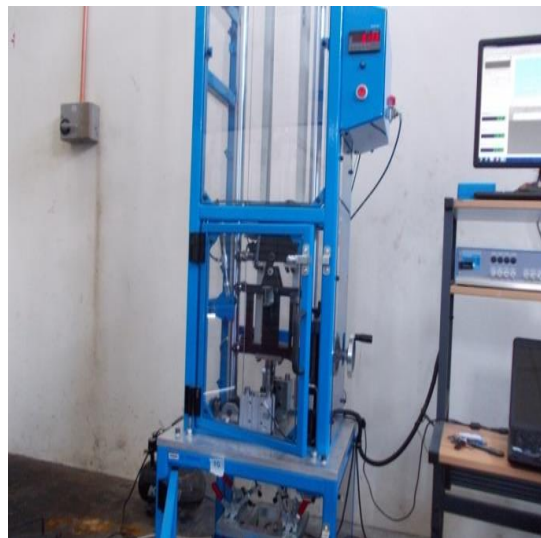
Fig. 5. Drop test for LVIT
