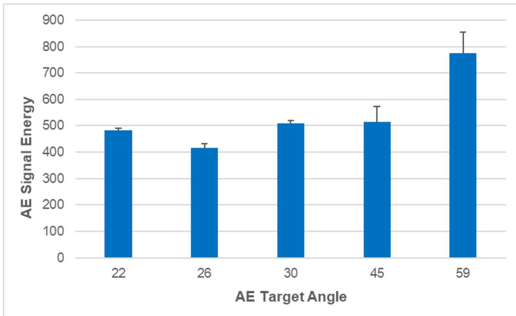
**Fig. 5.** Effect of AE target angle on AE signal energy (core material with 15% fines)
