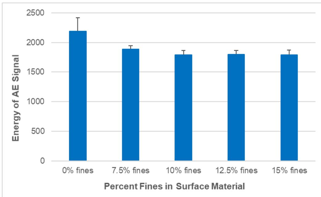
Fig. 7. Ability of AE system to detect fines in surface material (error bars = 1 standard deviation)
