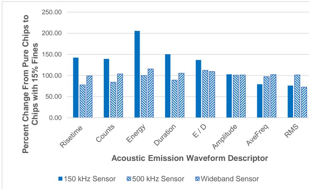
Fig. 3. Effect of acoustic emission sensor type and waveform descriptor
