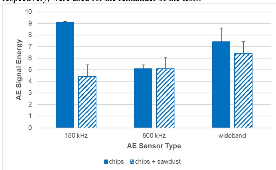
Fig. 4. Repeatability of “energy” waveform descriptor by sensor type (error bars = 1 standard deviation)
