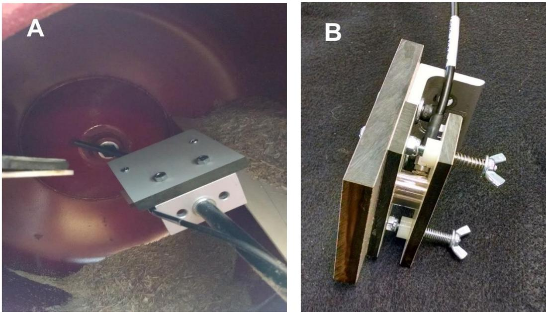
**Fig. 2.** (a) Inside of cement mixer used to tumble particles; (b) close up of AE sensor and target
