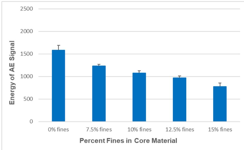
Fig. 6. Ability of the AE system to detect fines in core material (error bars = 1 standard deviation)
