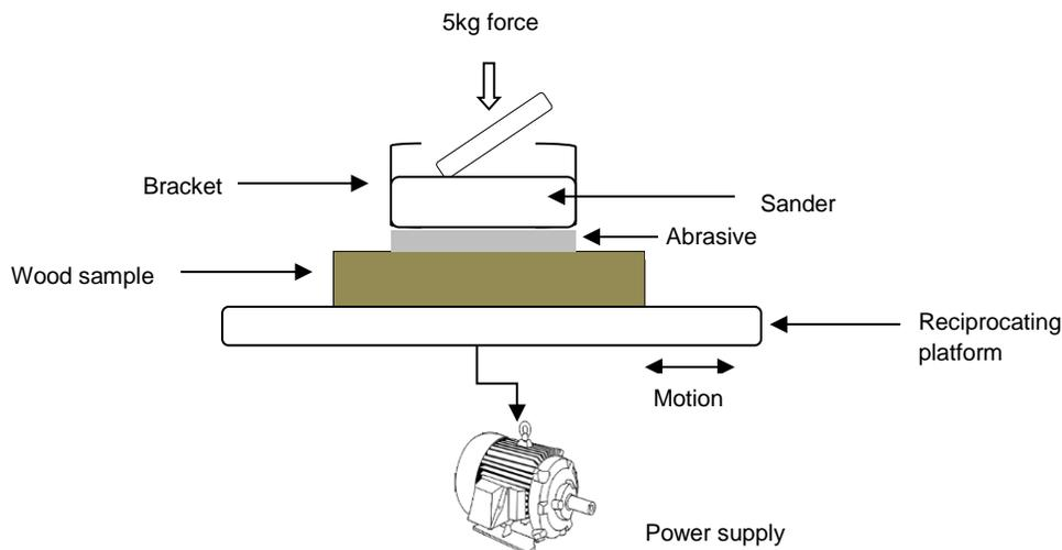
**Fig. 1.** Configuration of the abrasive sanding experimentation
