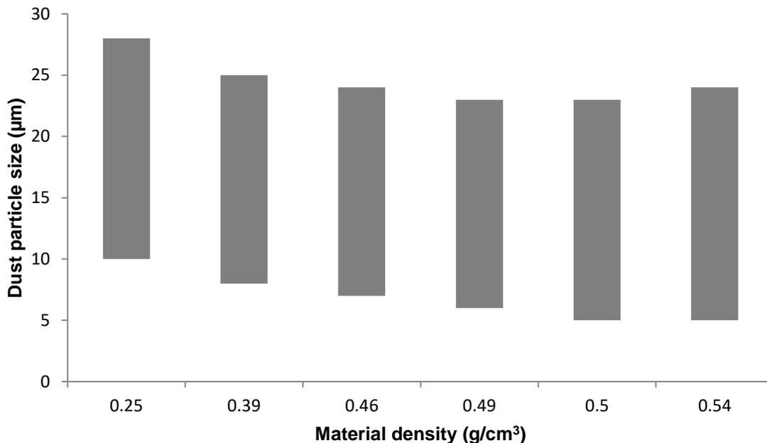
**Fig. 3.** Effect of wood density on range of dust particle size produced during abrasive sanding
