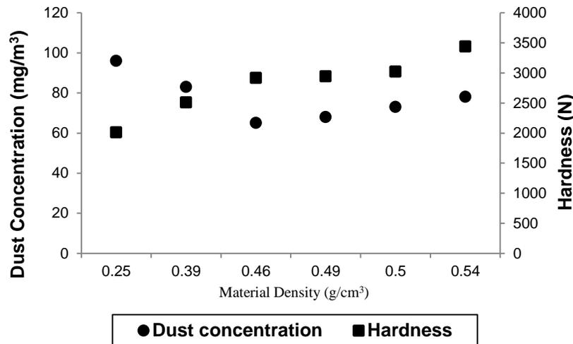
Fig. 2. Effect of hardness wood density on dust concentration
