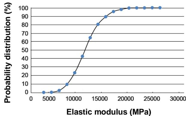
Fig. 3. Probability distribution diagram of elastic modulus of hemlock lumber
