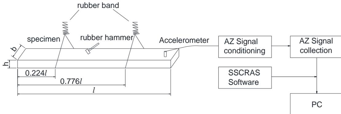
**Fig. 1.** Dynamic test block diagram of elastic modulus of lumber under free beam conditions
