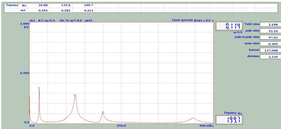
Fig. 5. Test spectrum of horizon of hemlock sawn timber specimens 12
