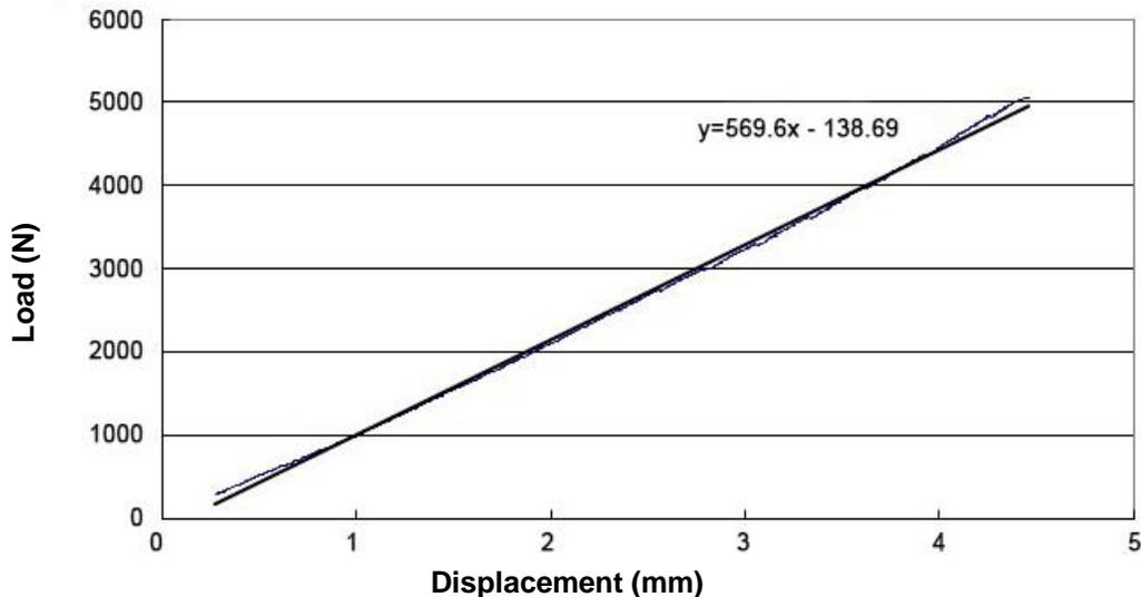
**Fig. 9.** CLT four-point bending test load displacement diagram
