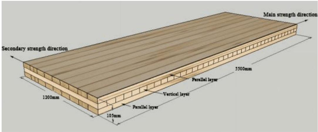
**Fig. 6.** Schematic diagram of CLT structure
