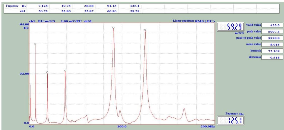
**Fig. 2.** Specimen 101 test spectrum of hemlock sawn timber
