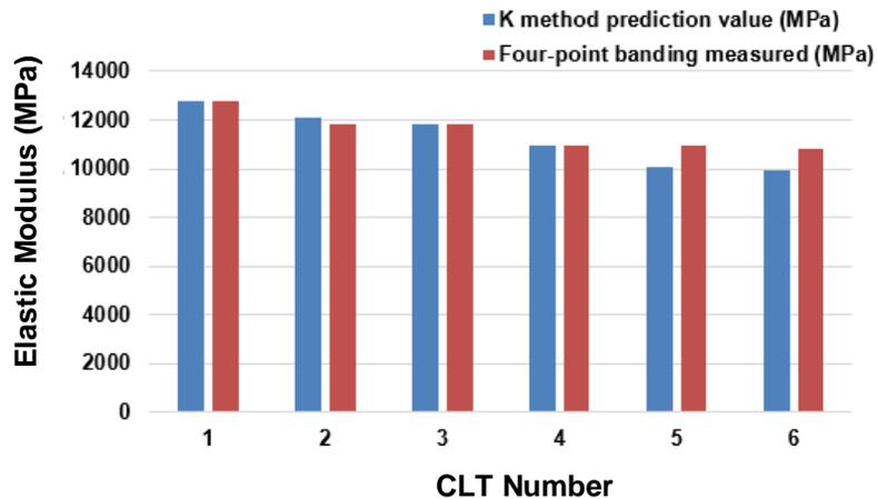
**Fig. 10.** Predicted and measured elastic modulus of CLT in primary strength direction
