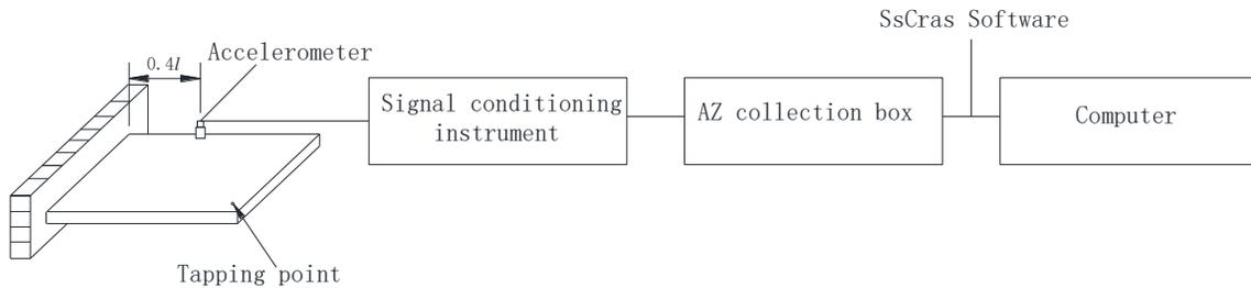
Fig. 4. Dynamic test block diagram of shear modulus of fir lumber under cantilever plate
