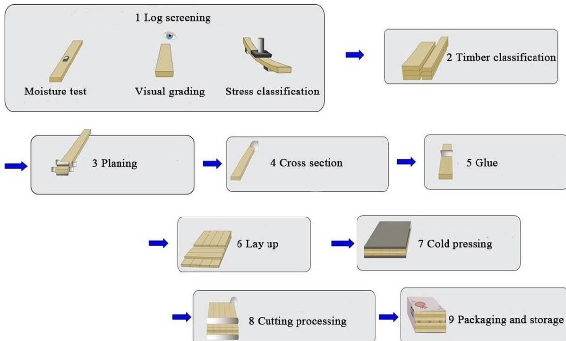
**Fig. 7.** CLT manufacturing flow diagram
