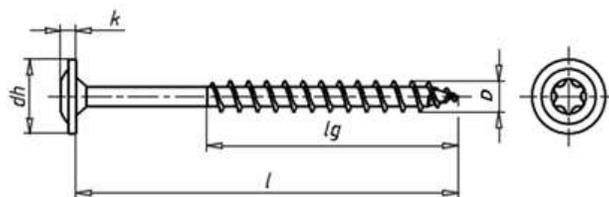
**Fig. 2.** Schematic diagram of the self-tapping screw (Würth 2016)
