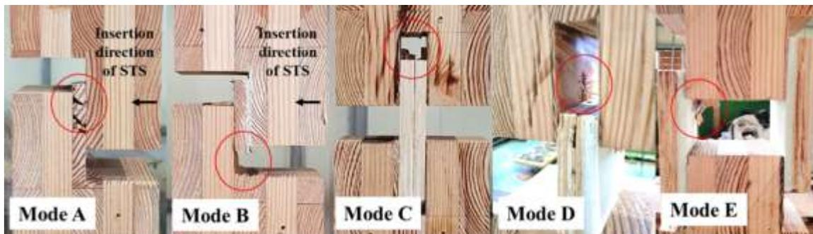
Fig. 10. Failure modes of the edge connections between the CLT panels
