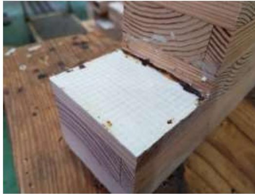
**Fig. 6.** Half-lapped connection reinforced with GFRP
