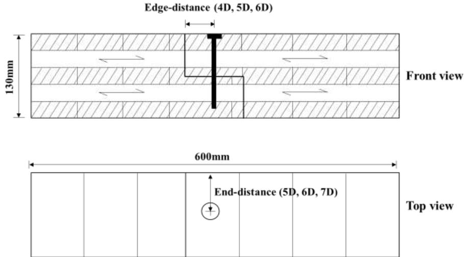
Fig. 3. Schematic diagrams of the half-lapped connection specimen
