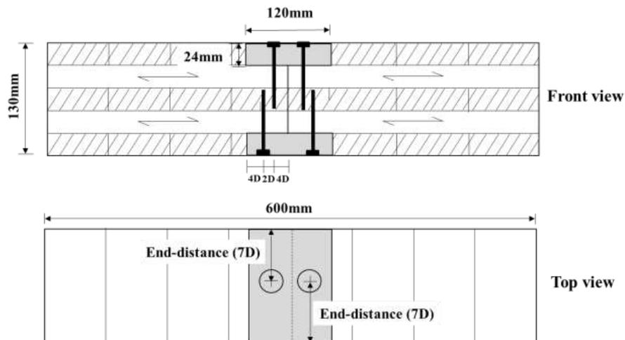
Fig. 5. Schematic diagrams of the double-spline connection specimen
