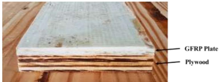
**Fig. 1.** Shape of reinforced plywood with GFRP plate
