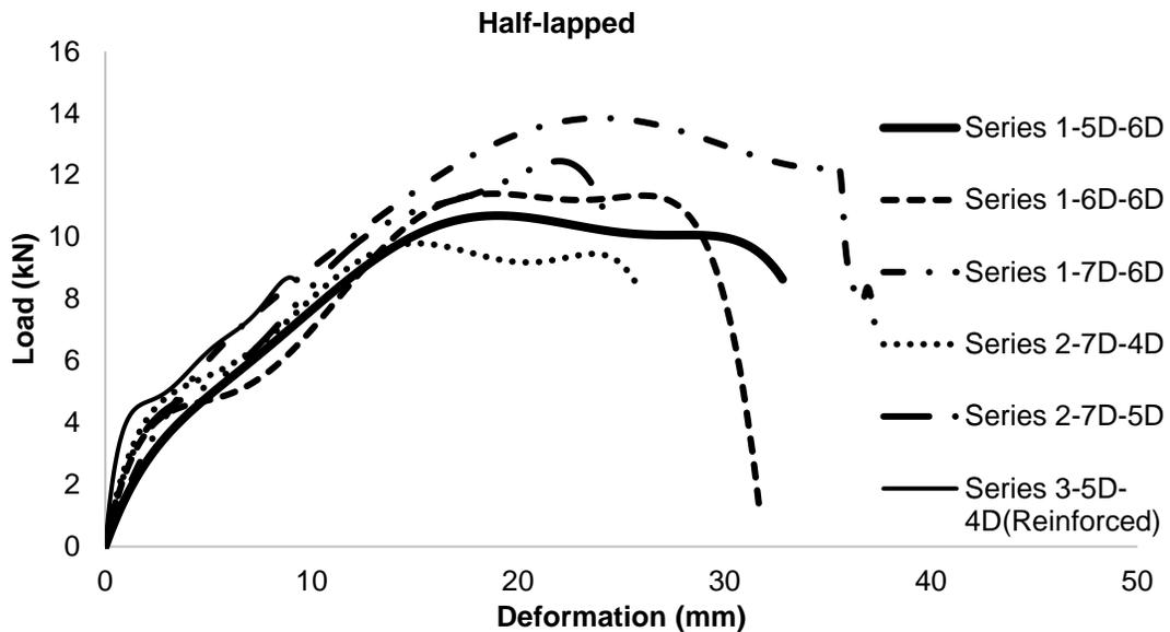
Fig. 8. Typical load-deformation curves of the half-lapped connection for the tension test
