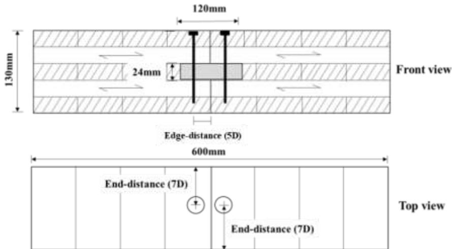
Fig. 4. Schematic diagrams of the internal spline connection specimen
