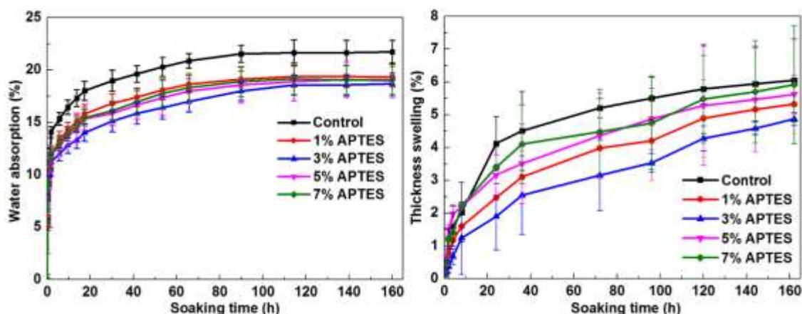
Fig. 10. Effects of fiber surface grafting on the water absorption properties of BF/PP composites
