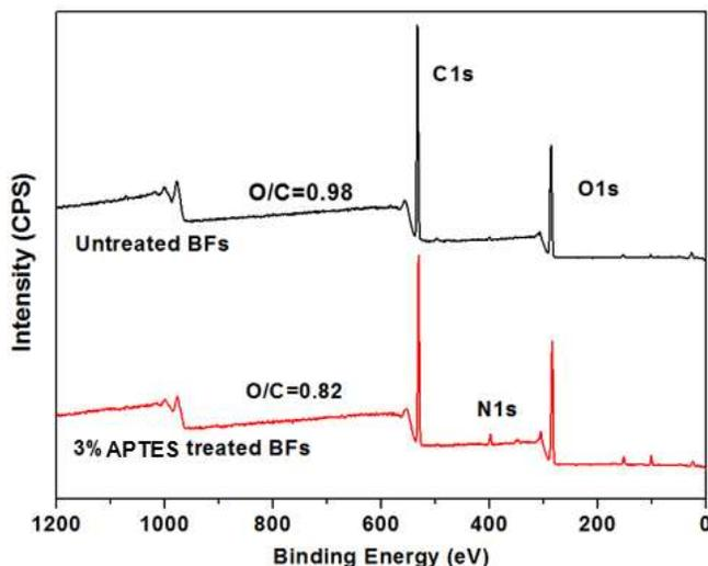
**Fig. 4.** XPS spectra of untreated BFs and treated BFs with 3 wt% APTES
