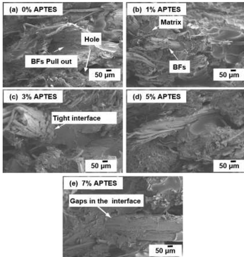
Fig. 8. SEM of fractured surface of BF/PP composites
