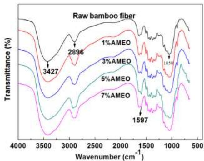
**Fig. 6.** FTIR spectra of raw BFs and treated BFs
