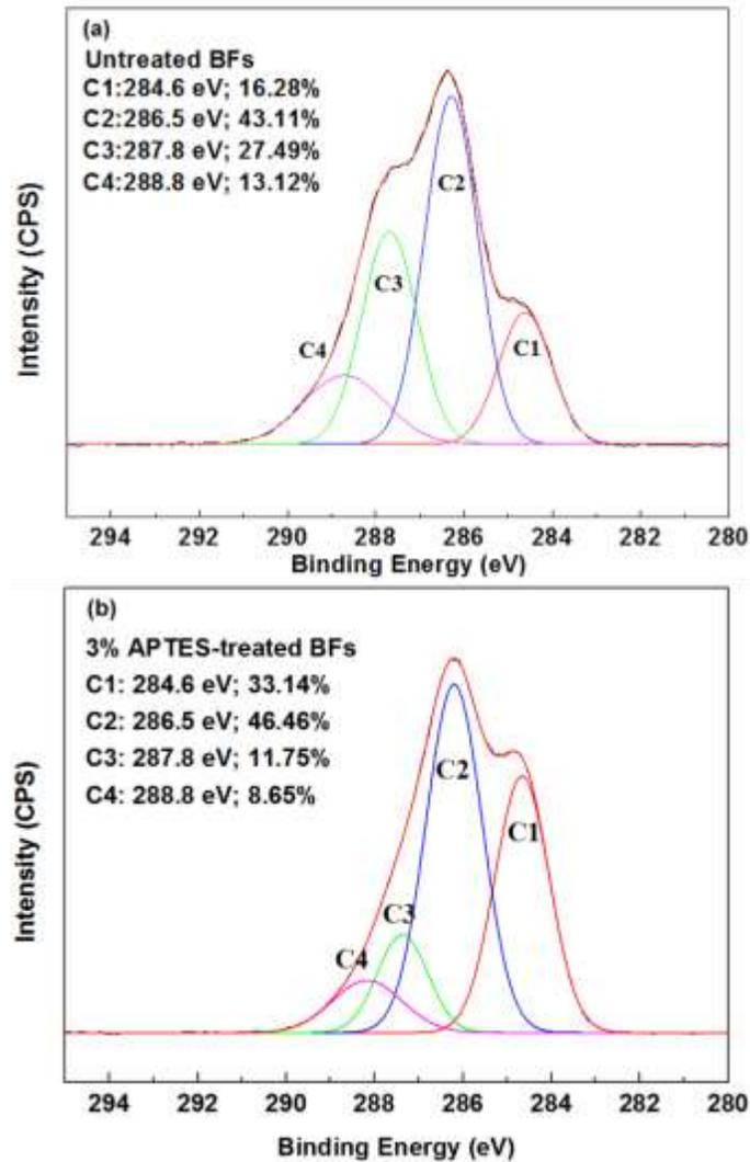
**Fig. 5.** High-resolution XPS C1 spectra of (a) untreated BFs and (b) BFs treated with 3 wt% APTES
