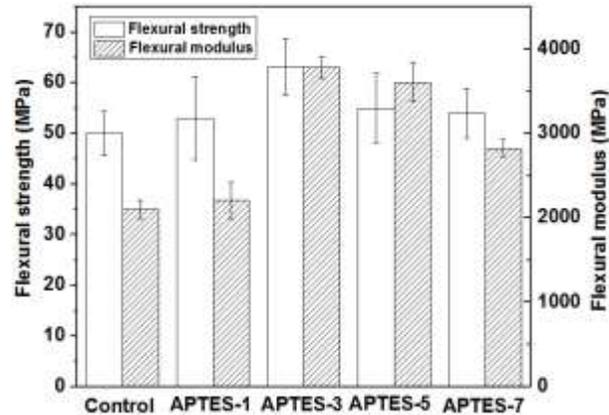
Fig. 7. Effects of fiber surface grafting on the flexural properties
