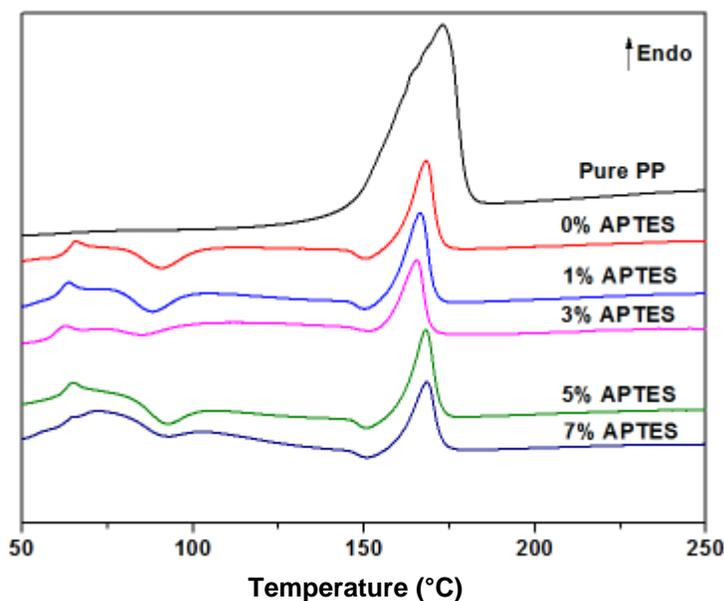
**Fig. 9.** DSC curves of pure PP and BF/PP composites
