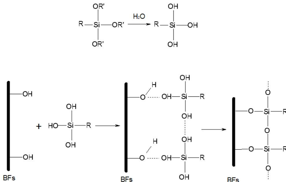
**Fig. 3.** The proposed chemical reactions between BFs and APTES
