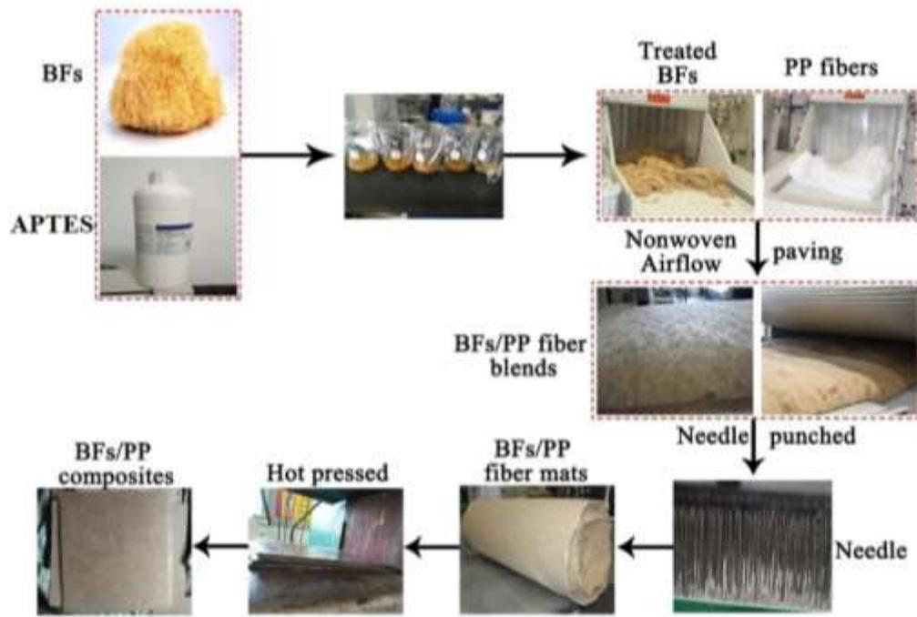
**Fig. 2.** Graphical illustration of the production process from BF and PP fibers to composites
